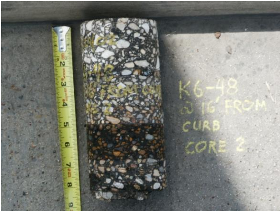
Figure 6.22. Intact Core Taken from Vicinity of K6-48.
