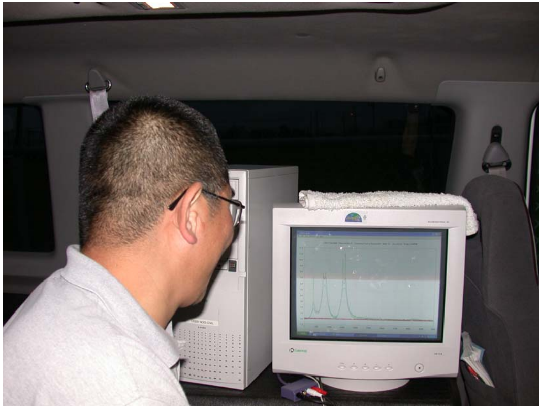
Figure B21. Monitoring and Recording MDD Displacements during Data Collection.
