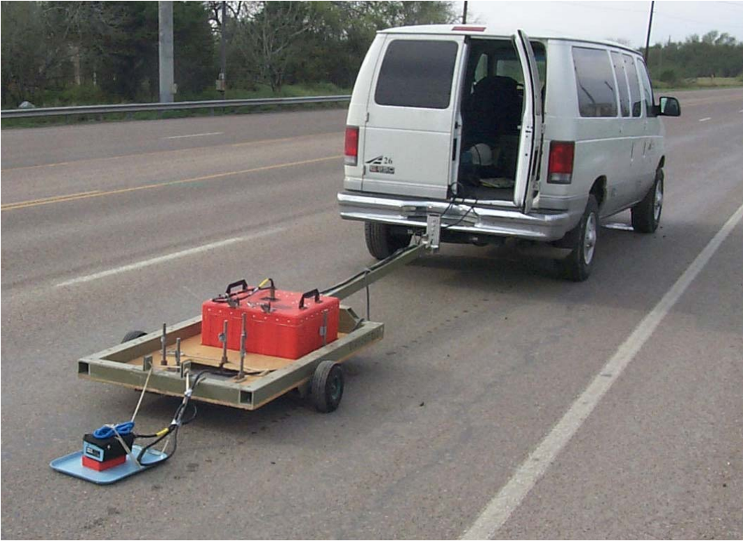
Figure 2.2. GPR Van with Ground-Coupled Antennas.
