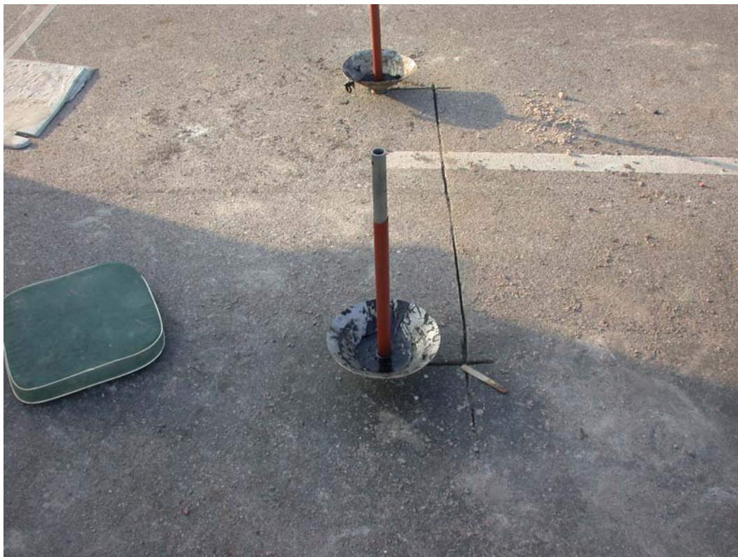
Figure B11. Curing of MDD Bonding Agent.
