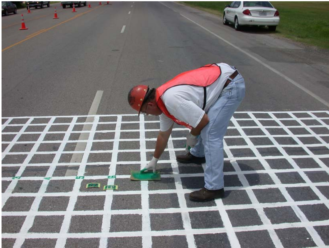
Figure B19. Grid Placed on Test Lanes for Determining Tire Placement.
