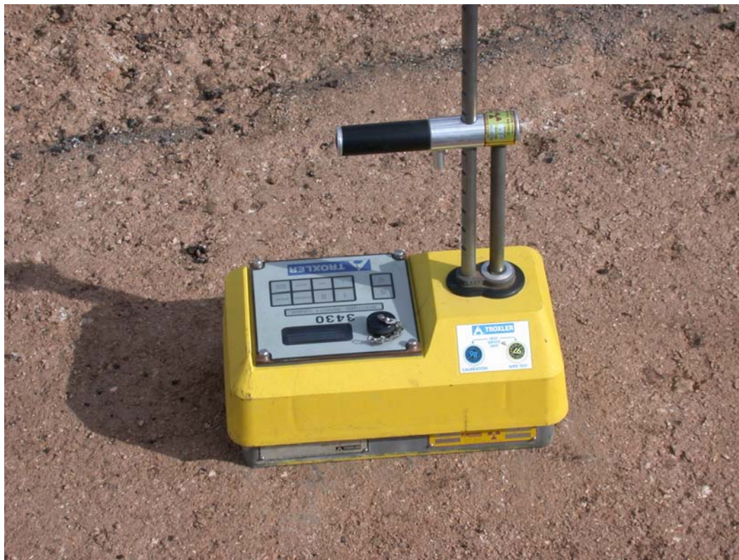
Figure B4. Density Measurement on Base Material.
