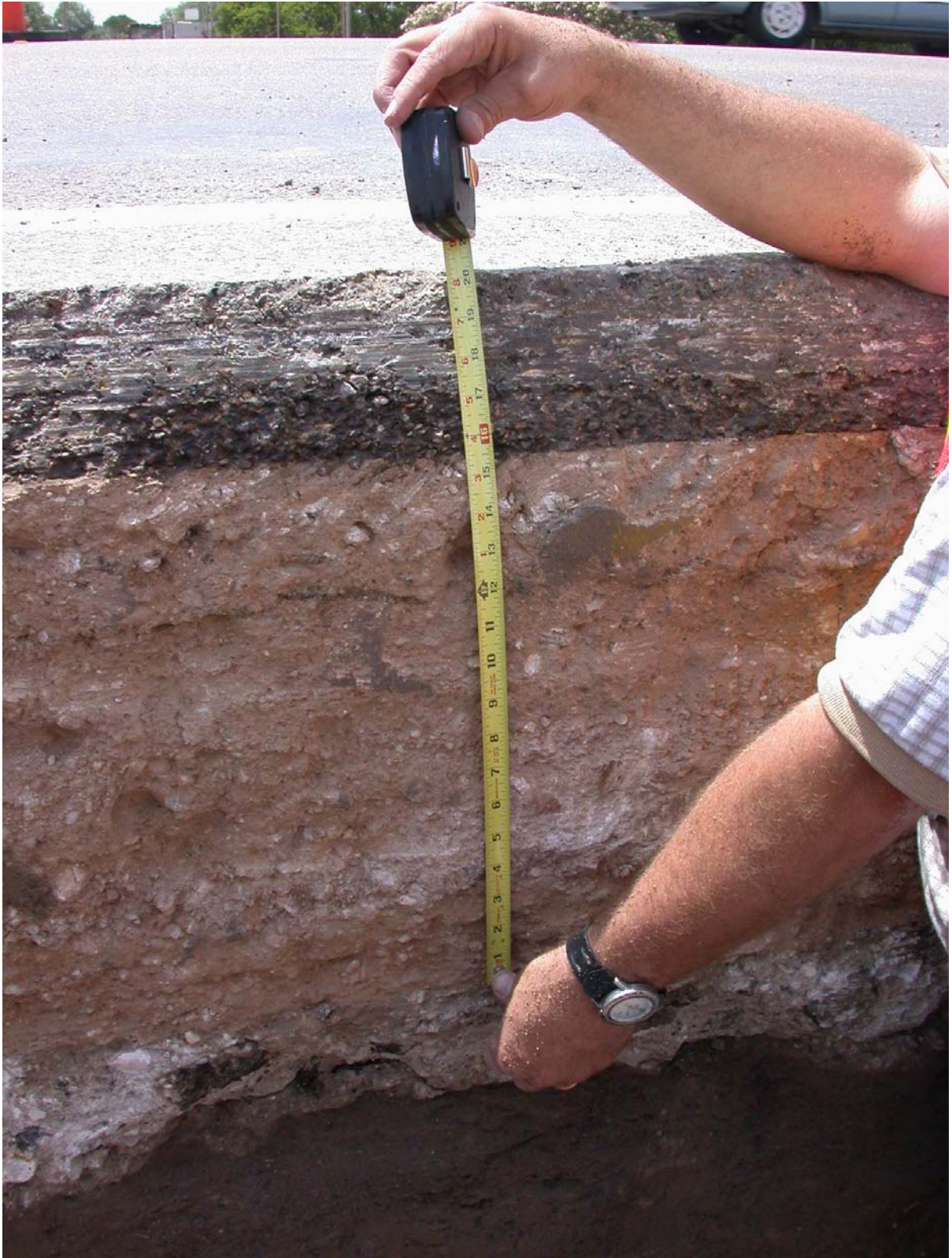
Figure B7. Establishing Depths of TDR Probes.
