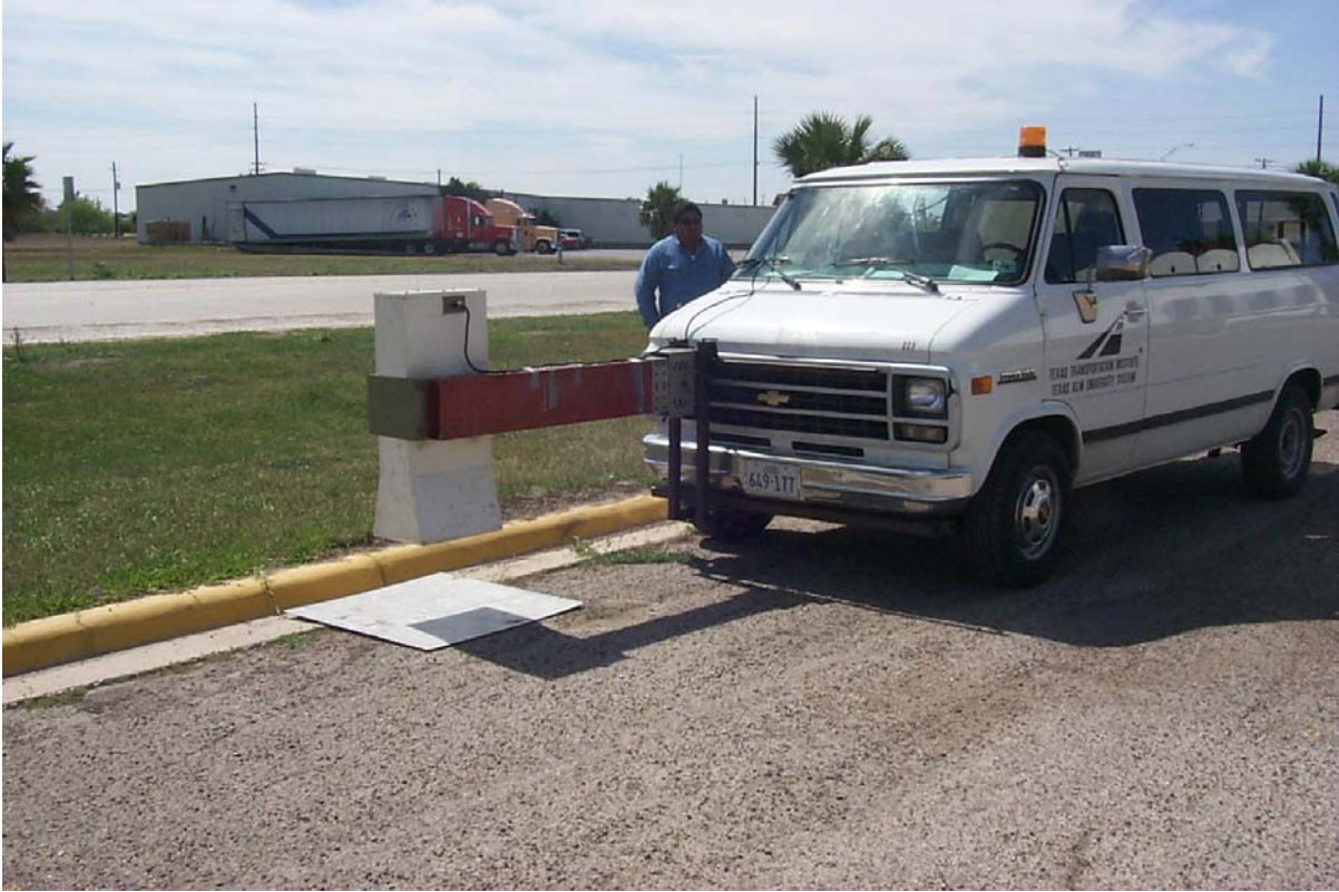
Figure 2.1. GPR Van with Air-Coupled, Front-Mounted Antenna.
