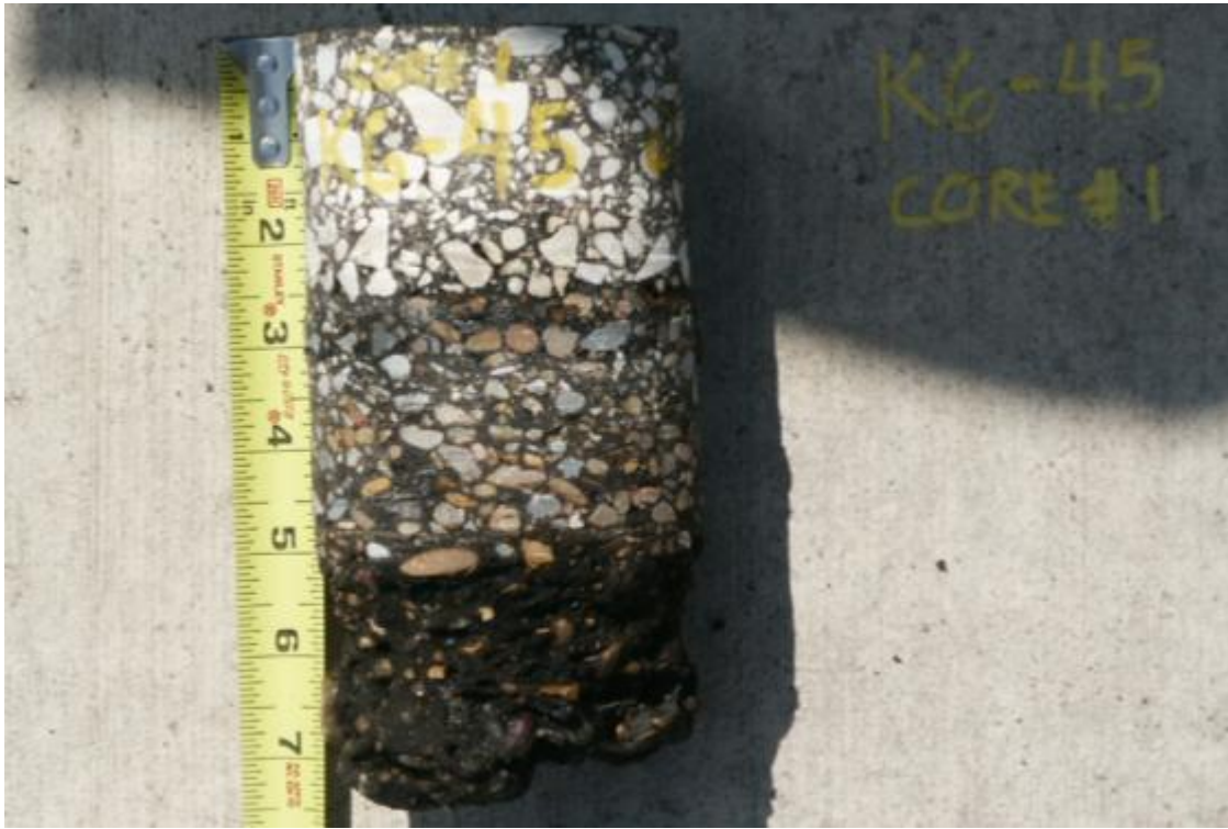
Figure 6.20. Piece of Broken Core Taken from Vicinity of K6-45.
