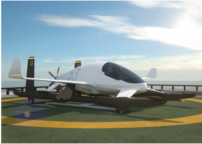
Aurora's eVTOL aircraft use eight lifting propellers for vertical takeoff, and a cruise propeller and wing to transition to high-speed forward cruise. (Aurora graphic)
