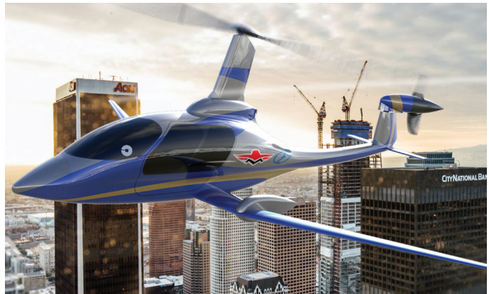
Carter and Mooney have teamed to develop the electric SR/C Air Taxi; the tail propeller rotates for forward thrust. (Carter graphic)
