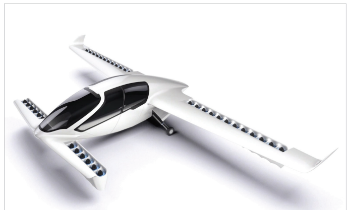
The new five-seat Lilium Jet design features a longer, fixed canard. For both lifting surfaces, the fans are mounted on split flaps that vector down for vertical lift. (Lilium photo)
