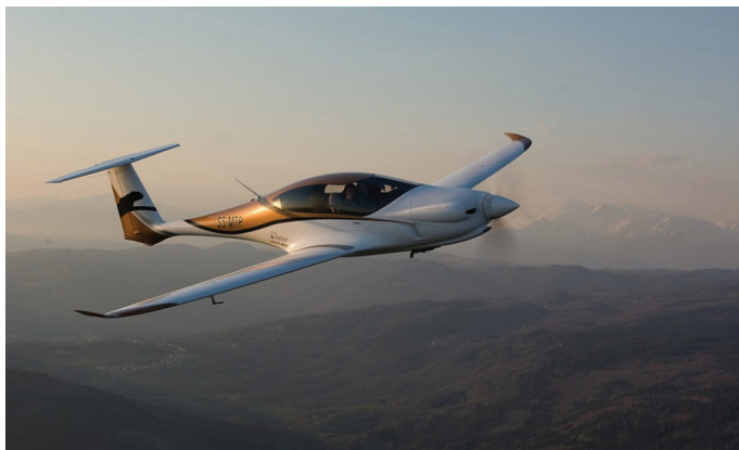
The non-VTOL Pipistrel Panthera is available with a piston/electric-hybrid: “Fly 4 people for 1000NM cruising at 200 KTS with 10 gallons per hour.” (Pipistrel photo)
