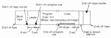
Fig. 12-13 Format of recorded cartridge tape. (RCA Broadcasting News.)
