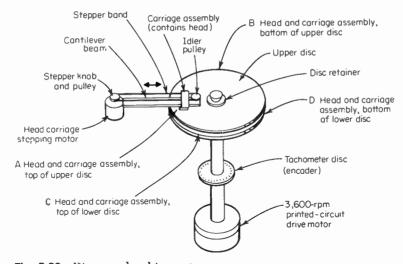
Fig. 8-22 Disc-recorder drive system.
