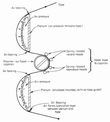
Fig. 8-4 Zero-loop drive system.
