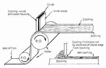
Fig. 6-5 Knife-blade coating process.
