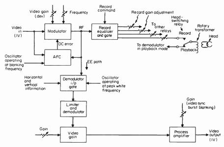
Fig. 11-12 Record-process block diagram.
