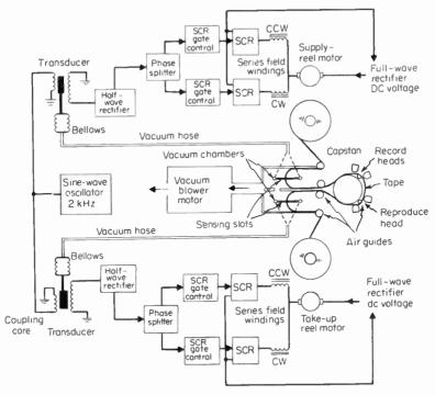
Fig. 8-32 Block diagram of reel servo using vacuum chamber.
