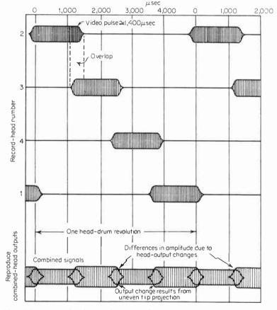
Fig. 5-8 Rotary-head recording/reproducing—signal recombination before correction.
