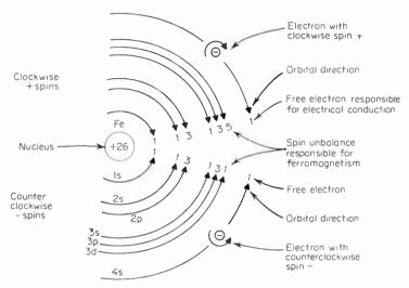
Fig. 4-1 Atomic structure of the iron atom.
