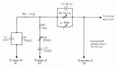
Fig. 9-8 Direct reproduce amplitude-equalizer schematic diagram.
