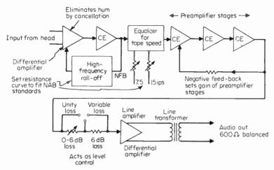
Fig. 9-3 Audio-reproduce and line amplifiers for video systems.
