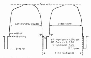
Fig. 11-16 The television signal—horizontal blanking.
