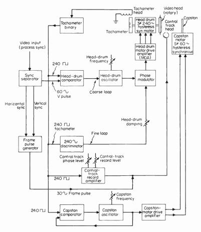
Fig. 11-6 Block diagram of record servo system.
