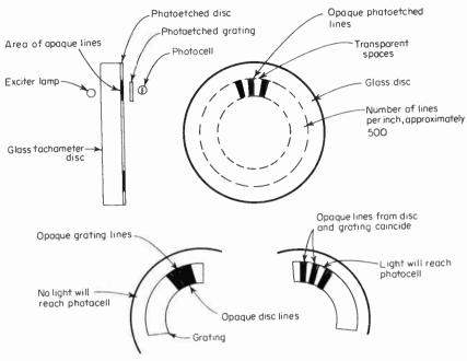
Fig. 8-7 Capstan tachometer system using photoetched disc.
