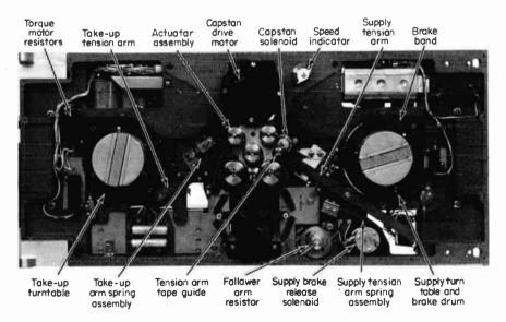
Fig. 8-36 CP 100 with overlay plates removed. (Ampex Corporation.)
