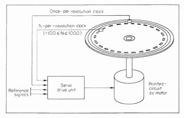
Fig. 8-28 Servo drive system. (Data Disc, Inc.)
