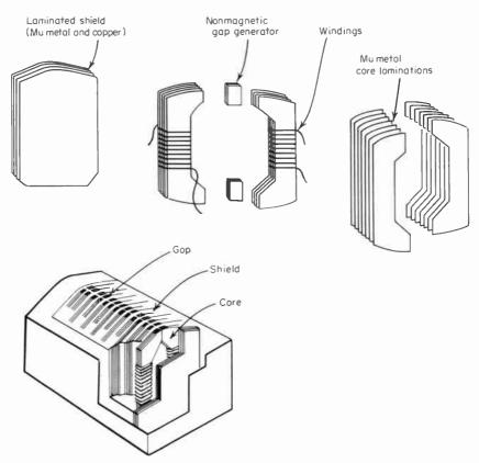
Fig. 5-3 Construction of a multitrack low-band magnetic head.
