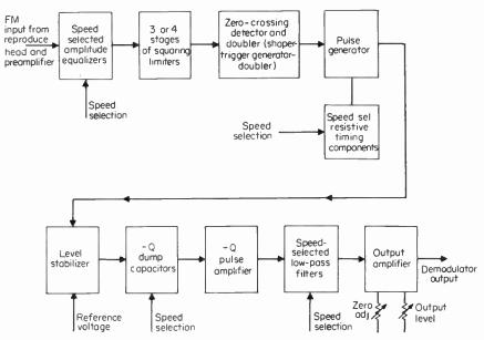
Fig. 10-9 Block diagram of FM demodulator-wideband group I multispeed.
