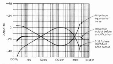
Fig. 7-24 Instrumentation amplitude equalization.
