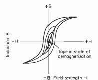
Fig. 3-3 The demagnetization curve.
