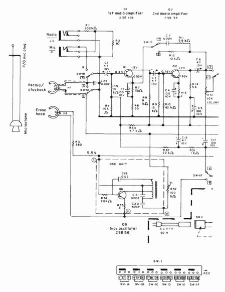
Fig. 12-5 Electrical schematic diagram of cassette recorder/player.
