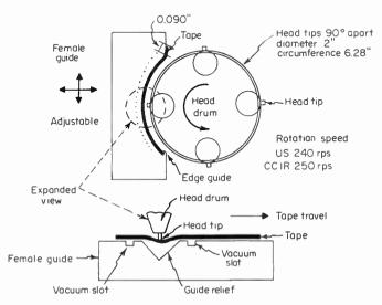
Fig. 11-1 Quadruplex-head- and tape-guiding details.
