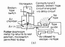
Fig. 8-40 Pneumatic brokentape sensing.
