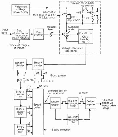
Fig. 10-10 Wideband group II multispeed, multiband modulator.
