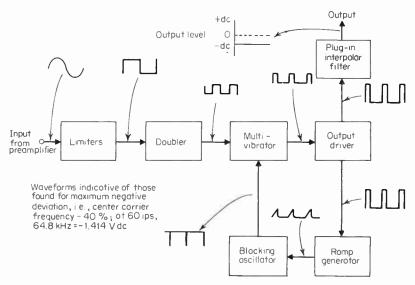
Fig. 10-5 Block diagram of type 2 FM demodulator.
