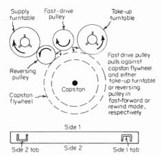
Fig. 12-9 Fast-mode operation—turntable-drive fast modes.
