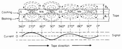
Fig. 7-1 Magnetic flux pattern on tape.
