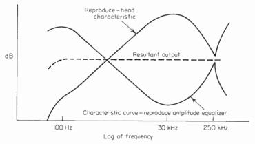
Fig. 3-6 Resultant of reproduce-head output plus amplitude equalization.
