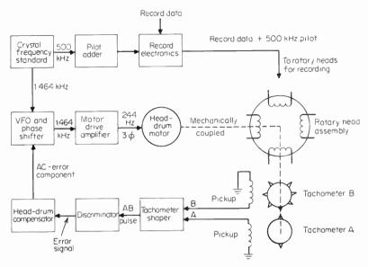
Fig. 8-13 Head-drum servo system—standard mode.
