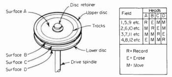
Fig. 8-24 Disc-surface lettering and switching format.
