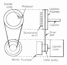
Fig. 8-6 Capstan tachometer system using slotted skirt.
