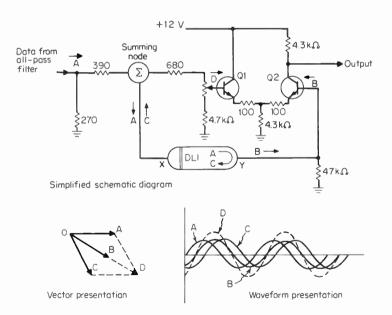
Fig. 9-16 Cosine equalizer—aperture-corrector action.
