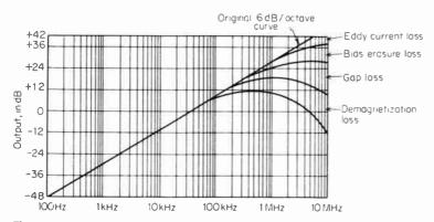
Fig. 7-15 Deviation from the 6 dB/octave reproduce curve due to losses.
