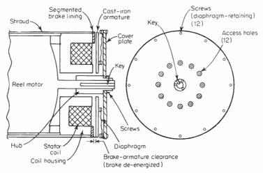
Fig. 8-34 Disc-type-reel motor brakes.
