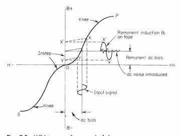
Fig. 7-8 DC-bias recording—method 1.
