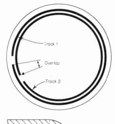
Fig. 8-25 Instrumentation discrecording overlapped tracks.
