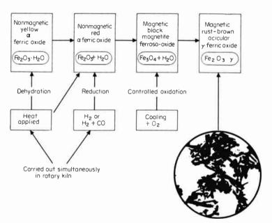
Fig. 6-2 Oxide conversion.
