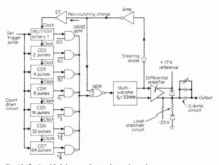
Fig. 10-13 Simplified diagram of recirculating charge dispenser.
