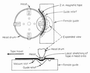
Fig. 5-9 Stretching of tape over rotary-head tips.
