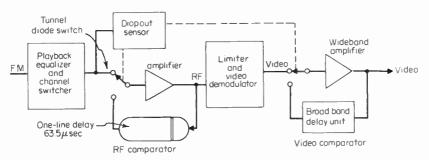
Fig. 11-18 Dropout correction using both RF and video correction.
