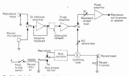
Fig. 9-1 Block diagram of a typical voice-log circuit.
