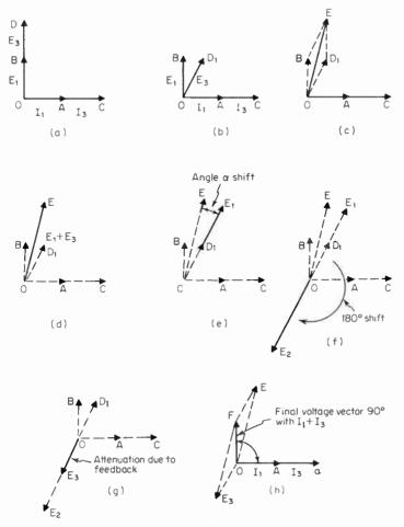
Fig. 9-10 Phase-equalizer vector diagrams.
