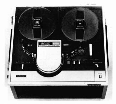
Fig. 8-16 AV 5000A Videocorder. This solid-state helical-scan color recorder uses 1-in. tape and a longitudinal tape speed of 7.5 ips and produces a tape pattern that conforms to the EIAJ Type I VTR Standard. (Sony Corp. of America.)
