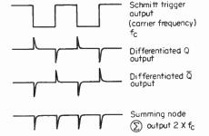
Fig. 10-3 Action of trigger-doubler circuit.
