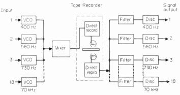
Fig. 1-2 Frequency-division multiplexing.
