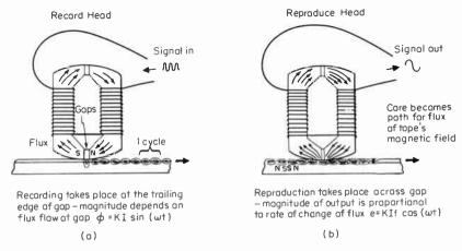
Fig. 5-6 Action at record and reproduce heads.
