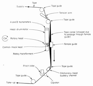
Fig. 8-10 Rotating-head (transverse-scan) drive system.
