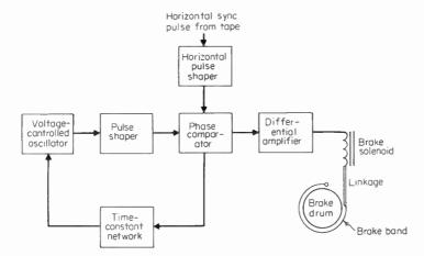
Fig. 8-18 Typical tape-tension servo system.
