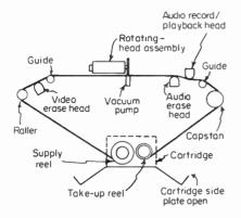
Fig. 12-12 Cartridge automatic-tape-threading path. (RCA Broadcasting News.)
