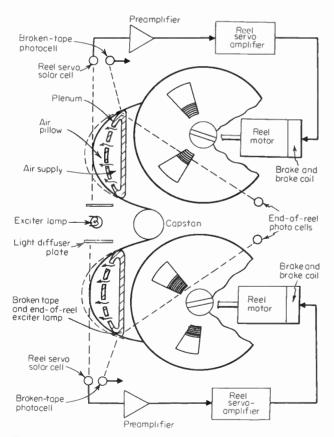
Fig. 8-33 Reel servo using plenum—simplified diagram.
