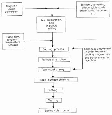
Fig. 6-1 Basic manufacturing processes of magnetic tape.
