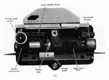
Fig. 5-7 Six-MHz rotary-head assembly—two-channel.
