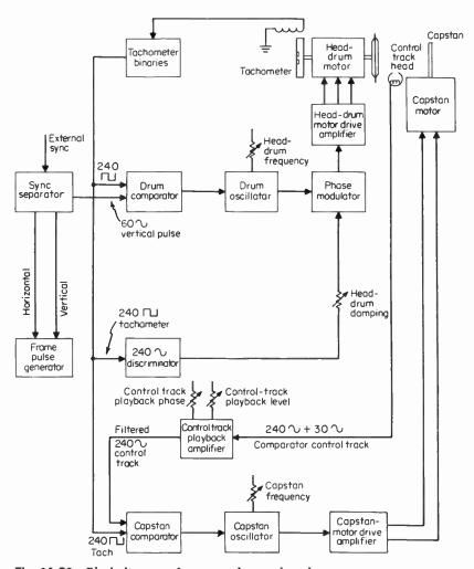
Fig. 11-20 Block diagram of preset and normal modes.
