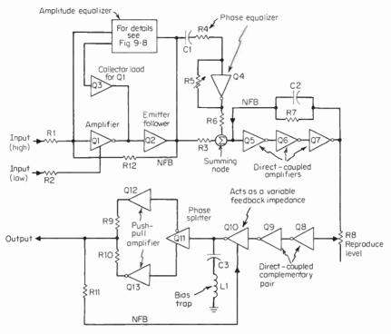
Fig. 9-7 Simplified diagram of single-speed direct reproduce amplifier.
