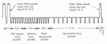
Fig. 11-7 A typical television vertical blanking pulse following an odd field.
