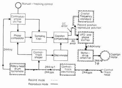
Fig. 8-12 Capstan servo systems—record and reproduce modes.
