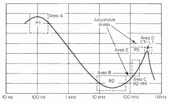
Fig. 9-9 Typical amplitude-equalizer curve.
