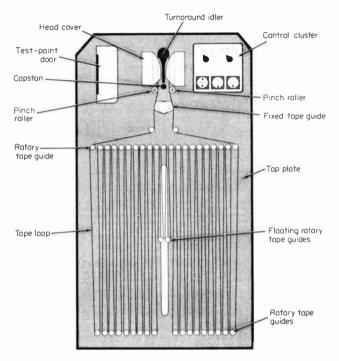
Fig. 8-30 Loop transport—tape-threading path.
