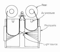
Fig. 8-31 Tape storage using vacuum and photoelectric sensing.
