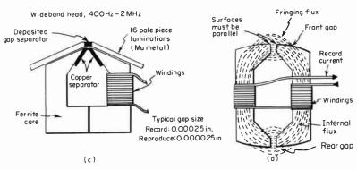
Fig. 5-1 Head-core design.
