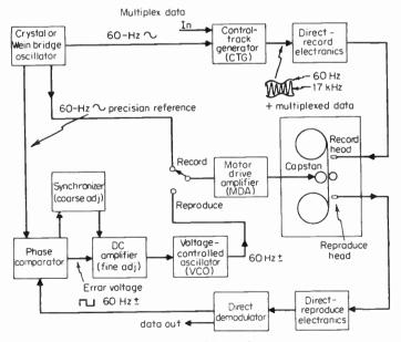
Fig. 8-8 A 17-kHz direct record/reproduce tape servo system.
