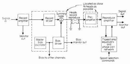
Fig. 9-12 Multiband 2.0-MHz-wideband direct system block diagram.
