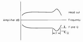
Fig. 11-15 Action of F-and-Q circuits.
