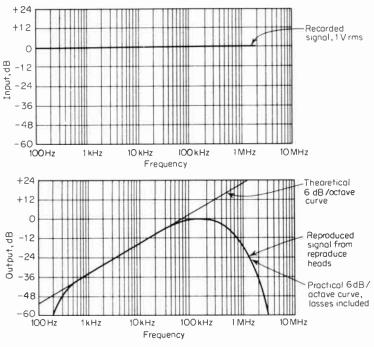
Fig. 7-23 The record and reproduce curves, indicating the need for equalization.
