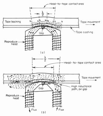
Fig. 7-21 Half-wavelength to head-contact-area ratio loss.
