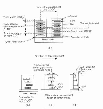
Fig. 5-4 Instrumentation head-stack parameters.
