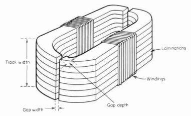
Fig. 5-2 Typical instrumentation head, low- and intermediate-band.
