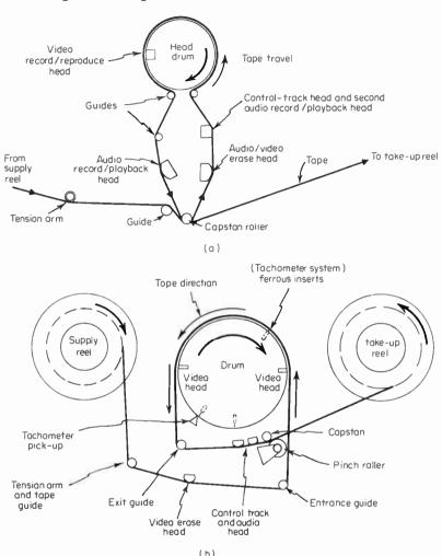
Fig. 8-15 Helical-scan drive systems. (a) Single-head system; (b) Dual-head system.
