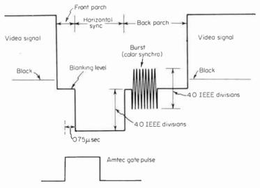
Fig. 11-19 Relationship of Amtec gate and edge of horizontal sync.
