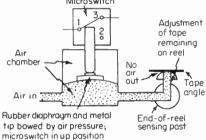
Fig. 8-38 Pneumatic end-oftape sensing. (a) Full reel of tape; (b) end of tape reached.
