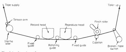
Fig. 8-1 Open-loop drive system.
