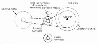
Fig. 12-8 Record and playback operation—turntable drive.
