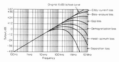
Fig. 7-20 6 dB/octave reproduce-head curve—high-frequency, short-wavelength losses taken into account.
