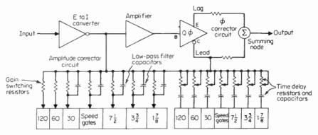
Fig. 10-12 Simplified diagram of amplitude- and phase-equalizer stages.
