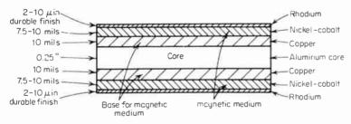
Fig. 8-20 Disc construction.
