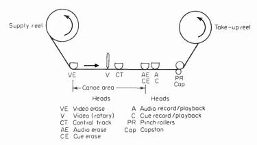
Fig. 11-4 The tape path of the quadruplex video recorders.
