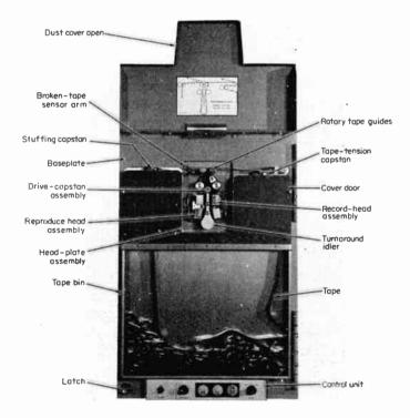
Fig. 8-29 FB 450 tape transport, front view. (Ampex Corporation.)
