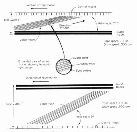
Fig. 8-17 Typical 1- and 2-in. helical-scan track patterns.
