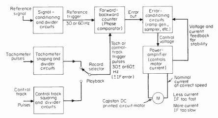
Fig. 8-19 Typical capstan servo system used with dc printed-circuit motors.
