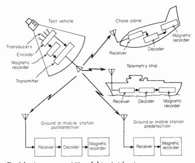
Fig. 1-1 Aerospace acquisition of data via telemetry.
