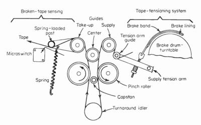
Fig. 8-39 Mechanical broken-tape and tape-tensioning systems.
