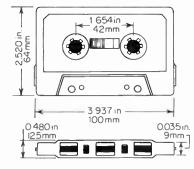
Fig. 12-3 The Philips cassette—dimensions.
