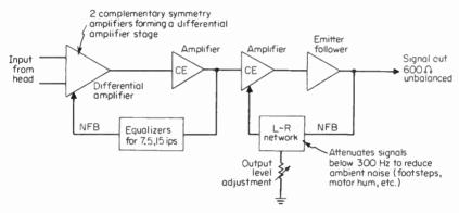
Fig. 9-4 Audio-reproduce amplifier for instrumentation.
