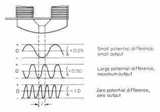
Fig. 7-14 Relationship of gap to wavelength.
