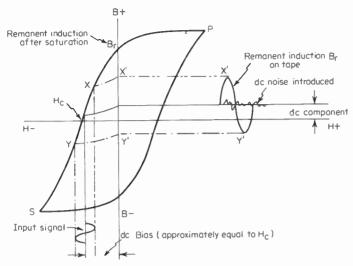
Fig. 7-9 DC-bias recording-method 2.
