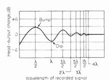
Fig. 7-22 Theoretical headbump curve.
