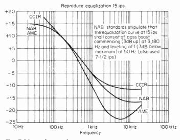
Fig. 7-26 Audio equalization curves.
