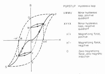
Fig. 7-4 Variations of magnetic induction B with magnetizing force H when H is less than that required to saturate the medium.
