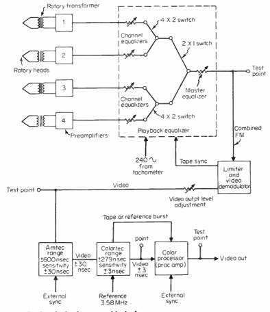
Fig. 11-14 Playback-process block diagram.
