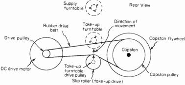
Fig. 12-7 Record and playback operation—capstan drive.
