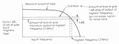
Fig. 7-11 Overbias setting for wideband recorders.
