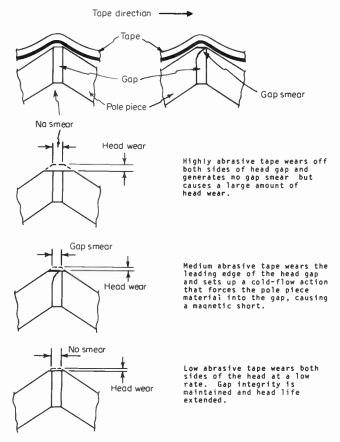
Fig. 6-7 Head-wear gap-smear problems.
