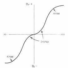
Fig. 7-6 Remanence flux vs. magnetizing force.  $B_r$ -H curve.
