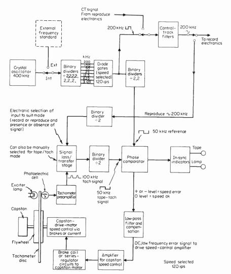
Fig. 8-9 A 200-kHz tape-speed servo system.
