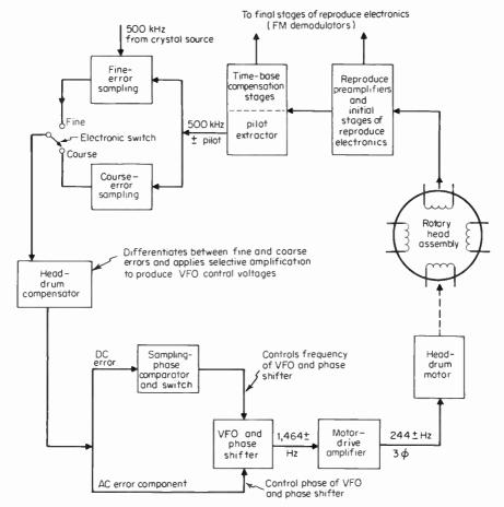
Fig. 8-14 Head-drum servo system—servo mode.
