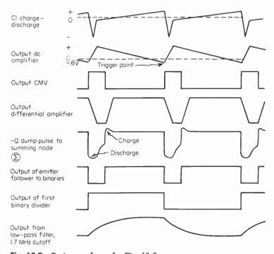
Fig. 10-8 Basic waveforms for Fig. 10-6.
