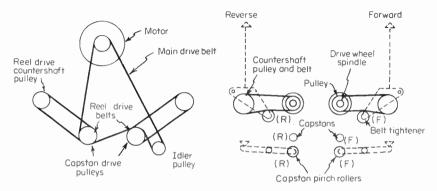
Fig. 12-11 Capstan-and-reel-spindle drive systems.
