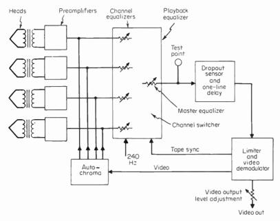
Fig. 11-17 Playback process with auto-chroma and dropout sensing.
