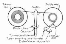
Fig. 8-37 End-of-tape sensing using follower arm.
