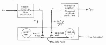
Fig. 3-1 The basic elements of a magnetic tape recorder/reproducer.
