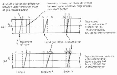
Fig. 7-16 Reproduce-head-azimuth error.
