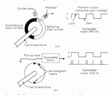
Fig. 11-5 Timing devices used to register head-drum speed.
