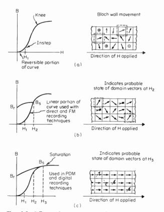
Fig. 4-2 Effects of a magnetizing force on a number of domains.
