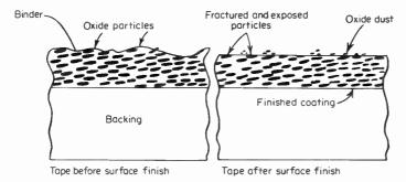
Fig. 6-6 Tape-surface imperfections left by some surfacing techniques.
