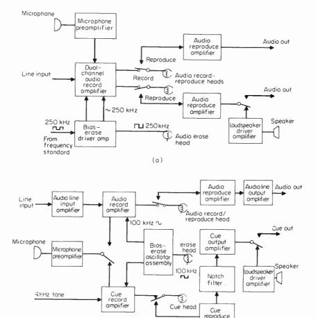
Fig. 9-2 Audio and cue block diagrams. (a) Rotary instrumentation and audio block diagram; (b) rotary video audio and cue block diagram.
