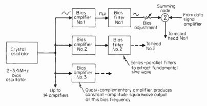
Fig. 9-6 Bias distribution system using master bias oscillator.
