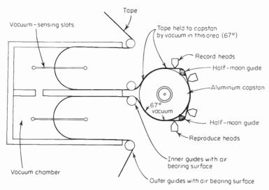
Fig. 8-3 Optimum-loop drive system.
