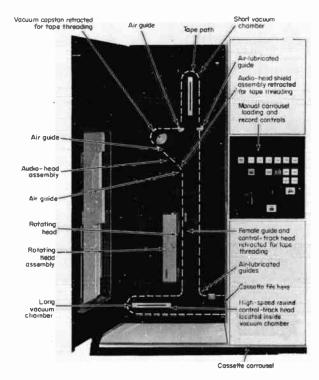
Fig. 12-16 ACR 25 tape-threading path. (Ampex Corporation.)
