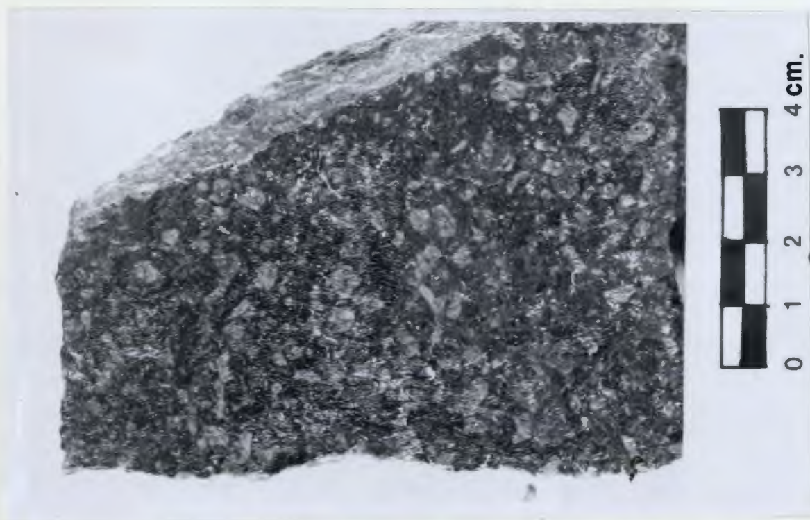
Plate 5: Pink euhedral feldspar phenocrysts in quartz-feldspar porphyry
