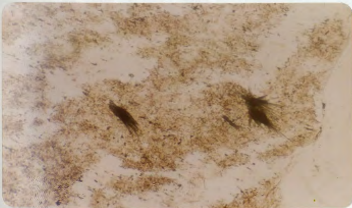
Photomicrograph 13: Clusters of riebeckite needles in feldspar (125 x)
