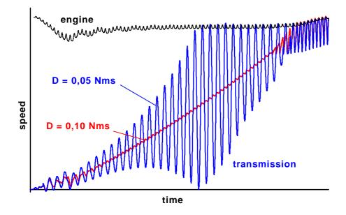
Figure 18: Consequences of different drive train damping based on the example of the facing chatter with  $\mu' = -0.010$  s/m (simulation)
