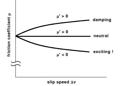
Figure 3: Principle friction coefficient curves
