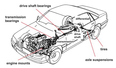
Figure 20: Transfer elements between drive train and vehicle body
