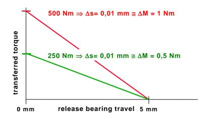
Figure 13: Clutch torque / release bearing travel dependence
