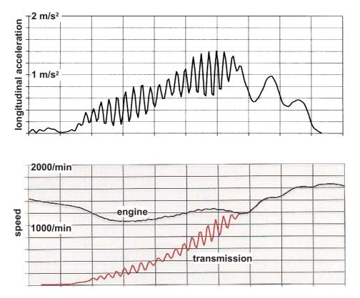
Figure 5: Forward vehicle acceleration (above), engine and transmission speed (below)
