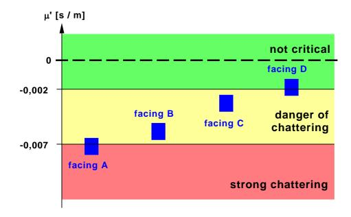
Figure 8: Friction coefficient gradients for different facings
