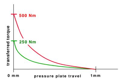
Figure 14: Clutch torque / pressure plate travel dependence
