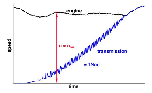
Figure 15: Chatter dependent on engine speed (measurement data)
