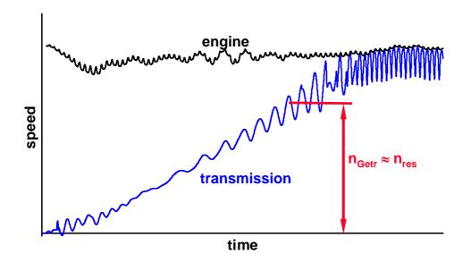
Figure 17: Chatter dependent on transmission speed (simulation)
