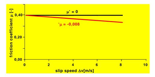
Figure 7: Friction coefficient curves
