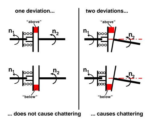
Figure 11: Model observation for pressure-induced chatter
