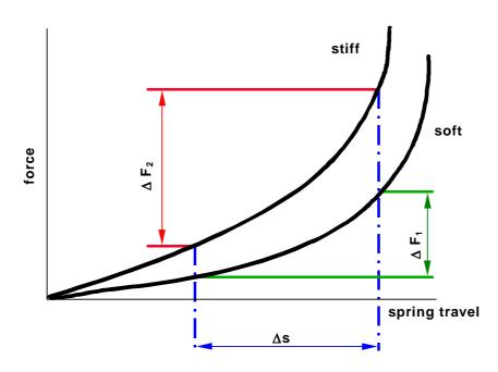
Figure 22: Friction facing curves
