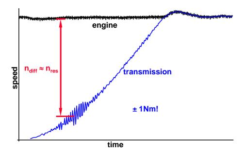
Figure 16: Chatter dependent on slip speed (measurement data)
