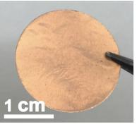
A copper current collector with a laser-induced silicon oxide coating created at Rice University. Courtesy of the Tour Group
