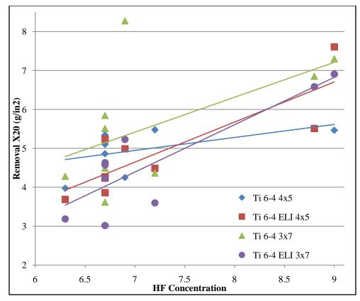
Figure 1: Metal Removal Comparison to HF Concentration
