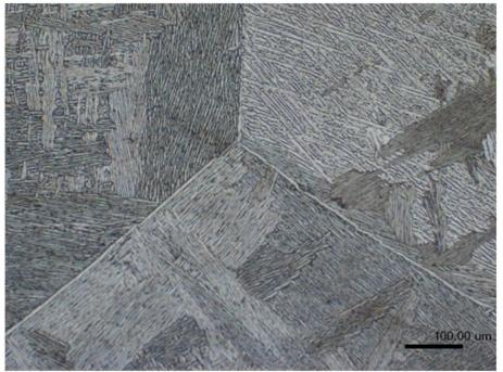
Figure 33:Ti-6-4 ELI, 10X Magnification
