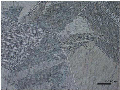
Figure 36: Ti-6-4, 10X Magnification
