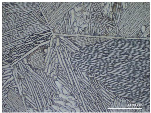
Figure 38: Ti-6-4, 20X Magnification
