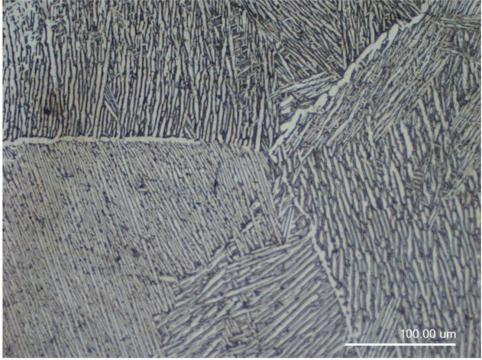
Figure 35: Ti-6-4 ELI, 20X Magnification
