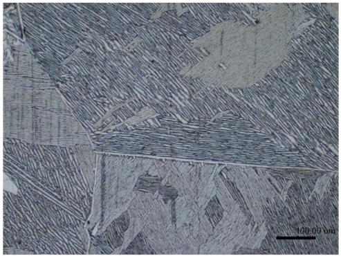
Figure 37: Ti-6-4, 10X Magnification, Second View
