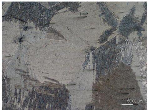
Figure 32: Ti-6-4 ELI, 5X Magnification
