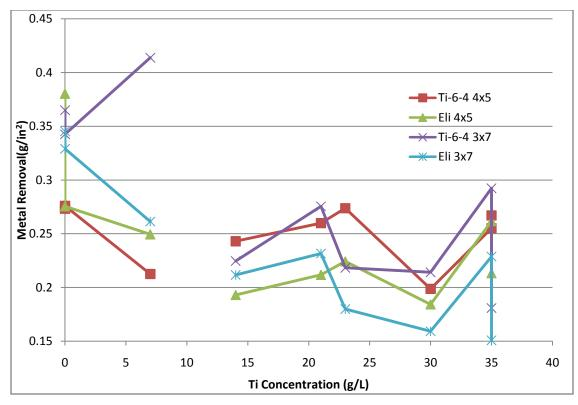
Figure 7: Metal Removal Dependence on Ti Concentration
