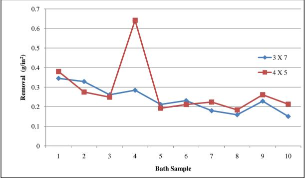
Figure 13: Weight Loss of Ti-6-4 ELI at Two Dip Times
