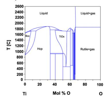
Figure 3: Titanium-Oxygen Phase Diagram (National Institute of Material Science, 2008)
