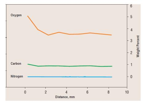
Figure 4: Oxygen Concentration in Titanium (Microstructure of Titanium Welds, 2004)
