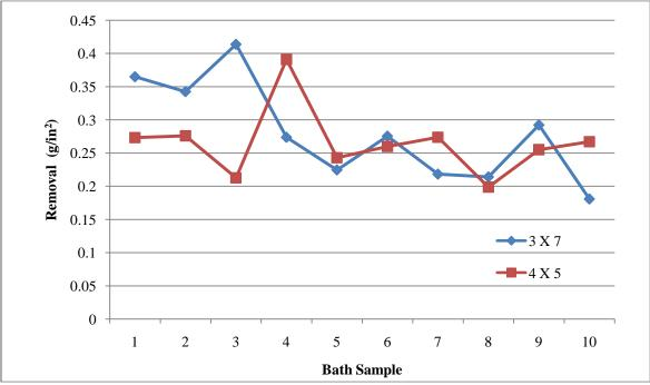
Figure 11: Weight Loss of Ti-6-4 Heated at Two Dip Times
