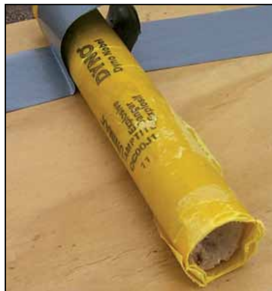
Figure 4.50 Explosives contain both an oxidizer and a fuel component in their chemical structures.
