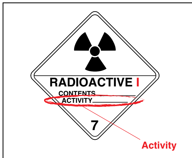
Figure 4.53 The activity of a radioactive source is listed on its radioactive label and represents the rate at which a number of atoms will decay and emit radiation in one second.
