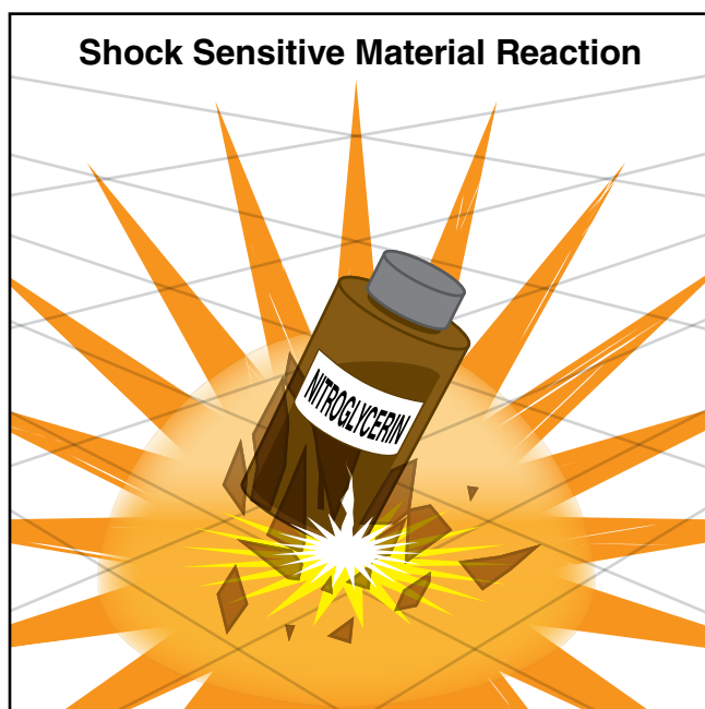
Figure 4.47 Shock- and friction-sensitive materials can be triggered into a violent chemical reaction by very little activation energy.
