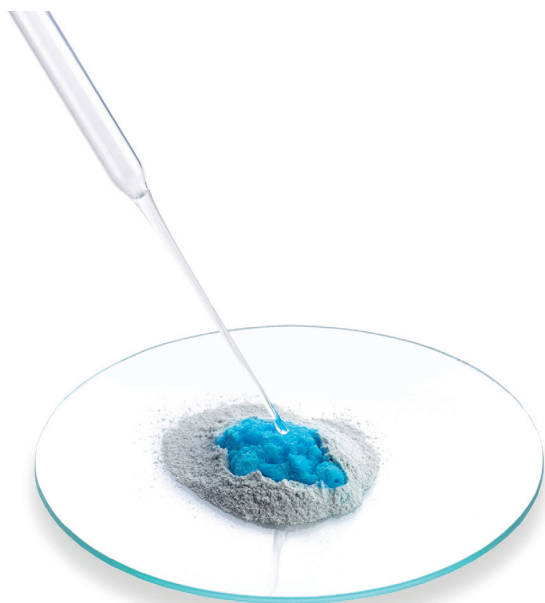
Water added to anhydrous copper(II) sulfate.
