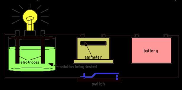
The ammeter measures the flow of electrons (current) through the circuit.
