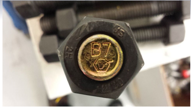
An ASTM A193, Grade B7 stud with an ASTM A194, Grade 2H Nut. The stud end is stamped B7 and the top surface of the nut is labeled 2H (raised letter and number)
