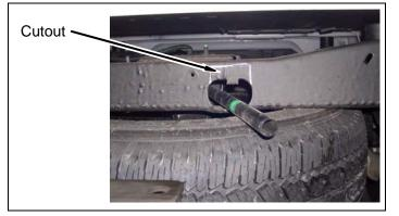
g. Install *kit* **bracket** (rear bumper, passenger) to rear bumper with factory hardware.
