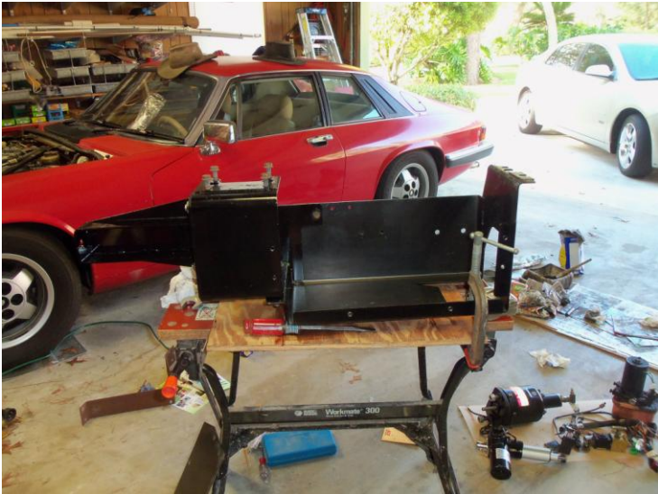
The reassembled unit housing after repainting has been completed. This is the access side, where the components were removed and the new components will be installed.
