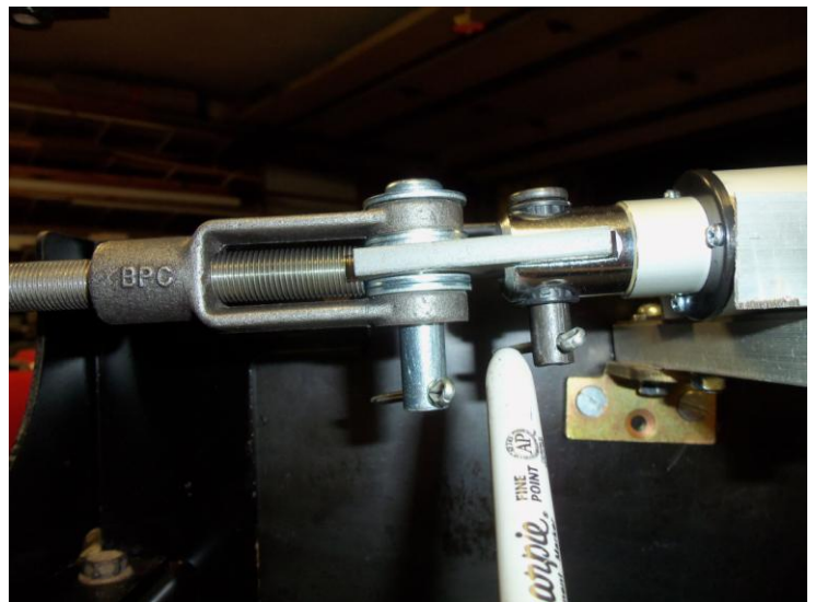
I made a steel flat-bar connector to go from the actuator mounting to the brake yoke.
