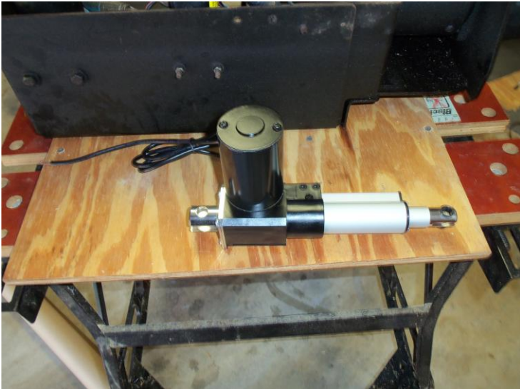
The parts in the previous photo are being replaced with this one part—a 12-volt DC linear actuator with a 3-inch stroke.
