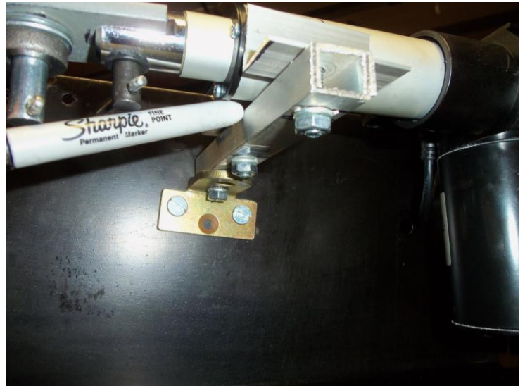
The linear actuator is resting on the bracket I made from two 3/4-inch aluminum channels. I used two holes already in the side of the box to mount the MB3; had to drill one hole out slightly, as the holes were not spaced exactly right.
