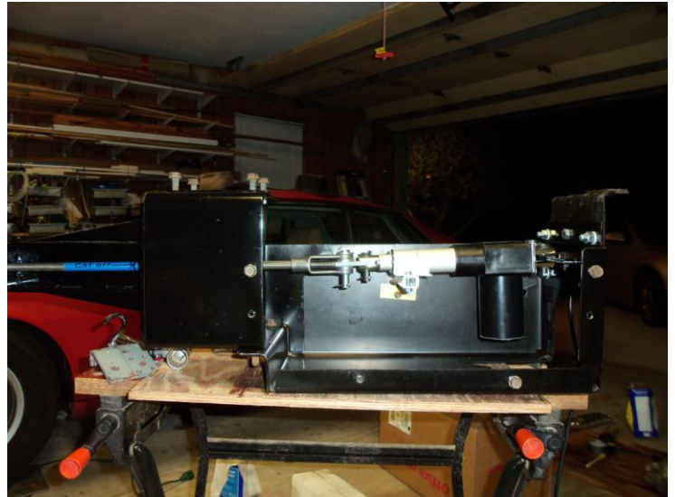
Side view showing how little is now in the box where all the hydraulic items were. Operation is now much less complicated and the unit is also much lighter.
