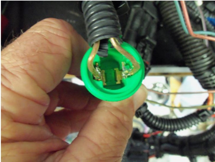
This is the RGS with the pressure section removed and wires soldered to the contacts.
