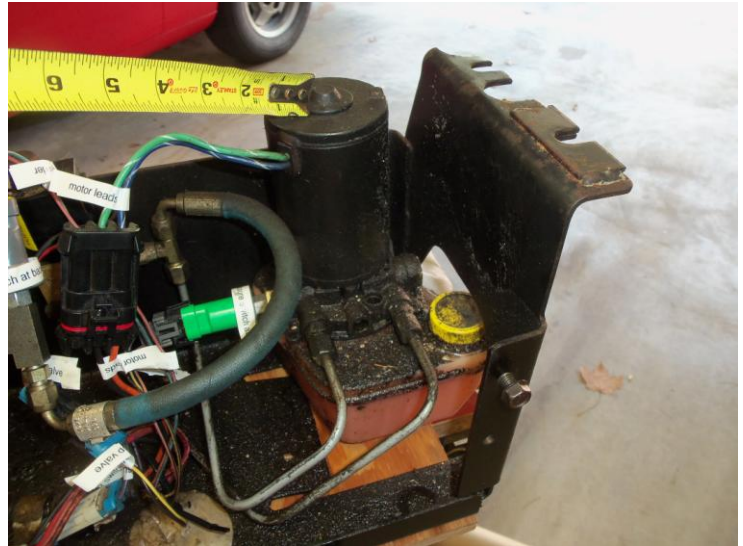
The hydraulic pump motor.
