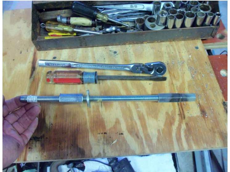
The tool I made to pull against the internal spring in the hydraulic cylinder to check the stroke length of the original park brake assembly.
