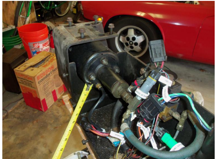
The hydraulic cylinder with the internal return spring.
