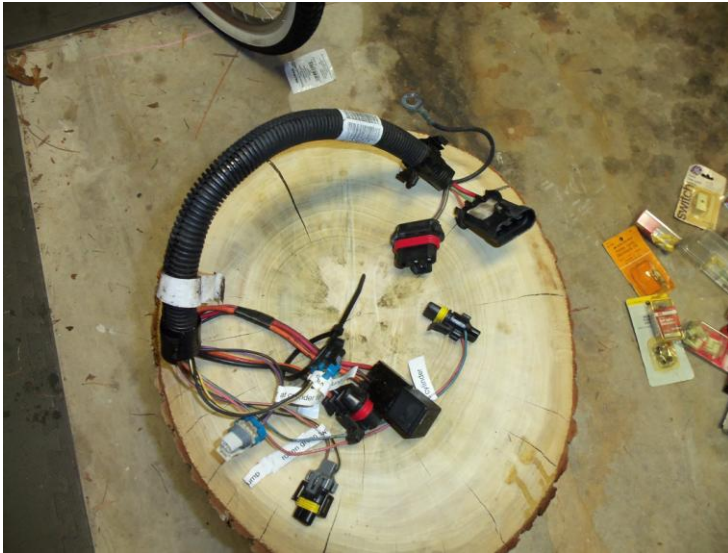
The factory wiring harness, which is part of the park brake unit. This is reused without alteration; the two connectors at the top of the harness connect to two connectors on the chassis, the ground connected to a bolt in the park brake unit housing.
