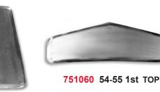
These cowl vent fillers are made a little larger than the stock vent opening so they can be trimmed for a good fit. Also, the outer edge has a slight roll to allow for a better flush weld. So, fill that hole & swap meet the old parts for a few bucks!
