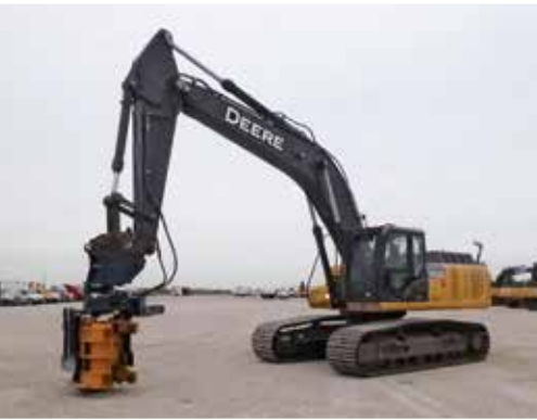
2013 John Deere 350G LC w/2018 Movax Sonic SideGrip SP-100
