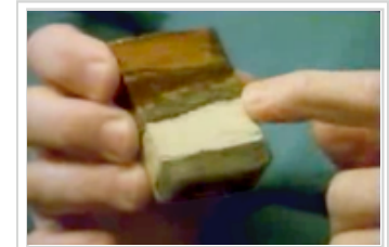
The piece of clay, held by Walter Alvarez, which sparked research into the impact theory. The second green band from bottom (third band up) is extremely rich in iridium.
