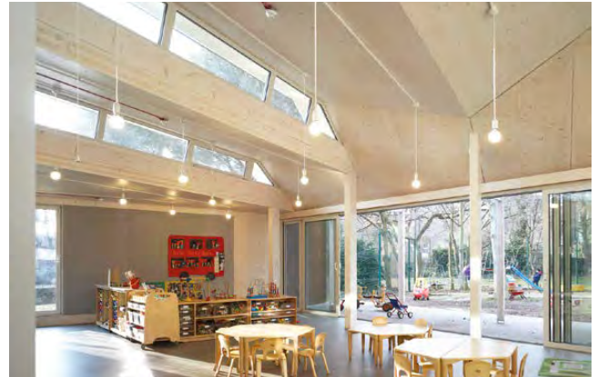
Clerestory windows are effective at adding natural light to activity rooms.
