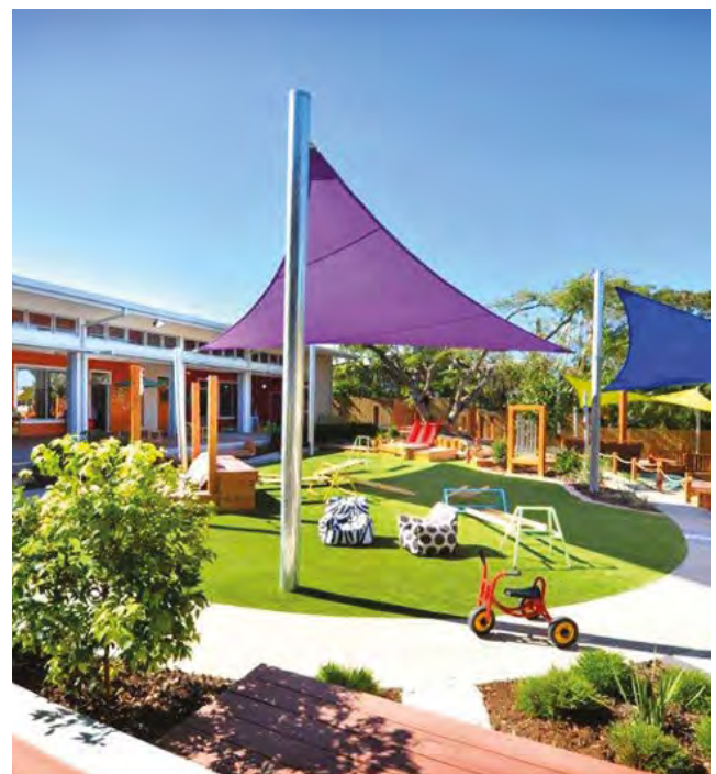
Shade structure can be a fixed structural element or a shade sail.
