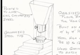
FLOUR BIN FOR "HOUR GLASS" BUILT ON A 4' by 4' PLATFORM TOTAL HIGH WOULD BE 10 to 12 FEET WOOD GRAINED WITCH'S CHAMB
