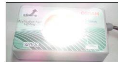
Final eRamp LED demonstrator: The area for power components can be reduced by a factor of about 3 using chip embedding in laminate technology
