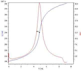
Fig. 2: Potentiometric determination of chloride in aqueous solution using the combined Ag-ring electrode (blue = measuring signal, red = ERC)
