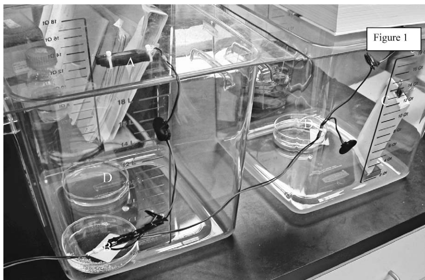
FIGURE 1. Treatment chambers with fan (A), dry FeCl_3 plus NaClO_2 in petri dish (B) or sachet (C), and aqueous solutions of KI as ClO_2 sinks (D).
