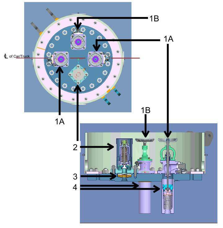
3.3 ALTERNATE VALVE DESIGN ARRANGEMENT – 4 LOADING/UNLOADING VALVES
