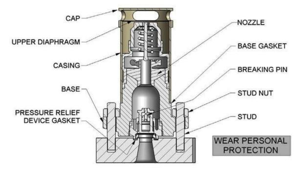
Figure 5.2 – Chlorine Pressure Relief Device (Traditional)
