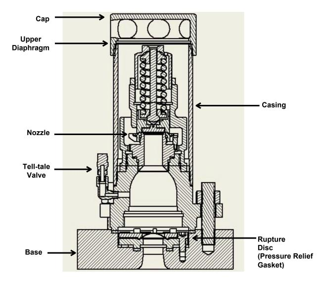
Figure 5.3 – Chlorine Pressure Relief Device (Alternate Design)
