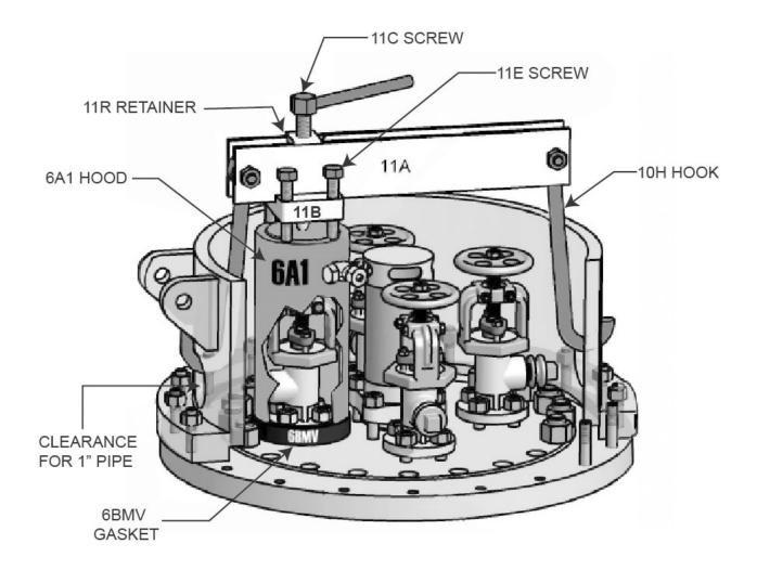
**Device 6 Assembled Over Angle Valve**
