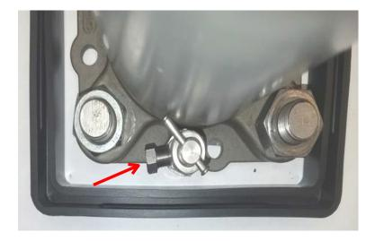
Figure 7.3 – Rotated tell-tale valve so it does not interfere with Hood 24A footprint
