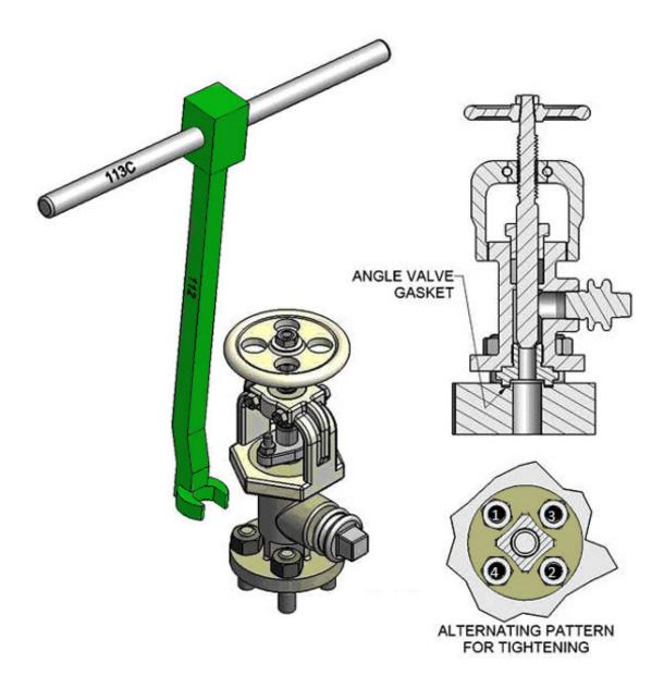
Figure 4.2 – Angle Valve Gasket Leaks and Required Tools
