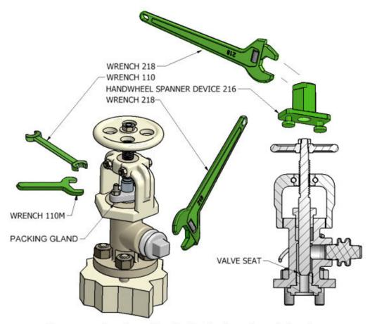
Figure 4.1 – Angle Valve Packing Gland Leak Points and Required Tools
