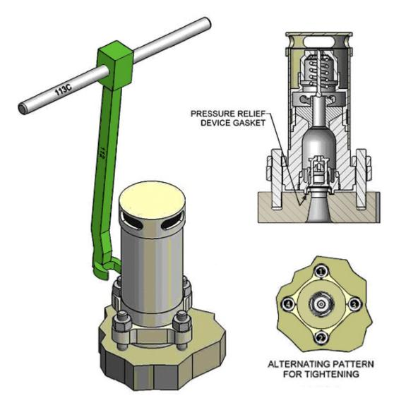
Figure 4.3 – Pressure Relief Device Leaks and Required Tools
