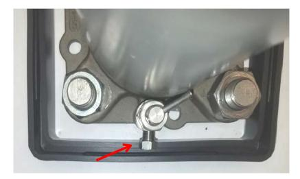
Figure 7.2 – Tell-tale valve plug shown extending into the Hood 24Afootprint
