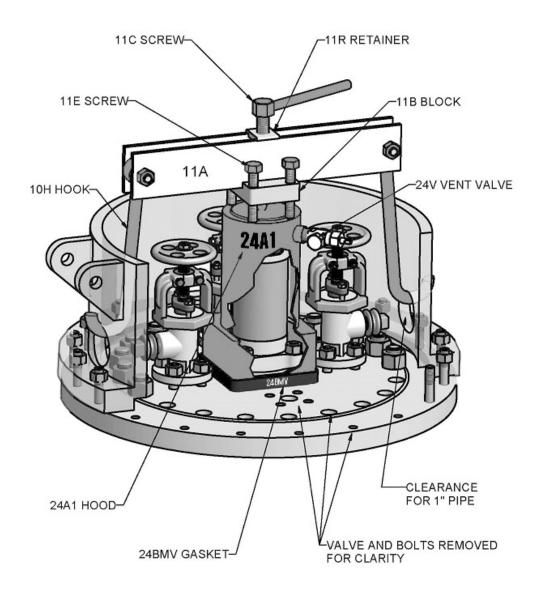
**Device 24 Assembled Over Pressure Relief Device**
