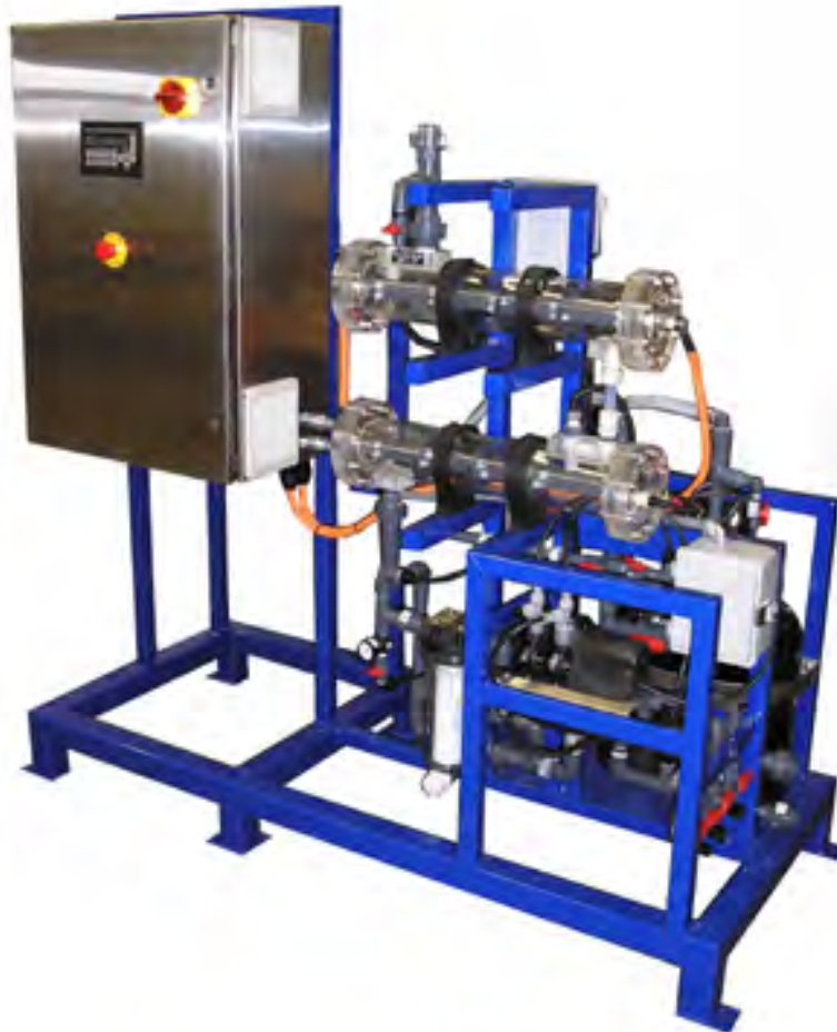
Typical 24 lb On-Site Hypochlorite Generation System
