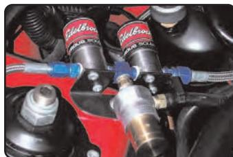
EFI Dry Nitrous Kit #70400 installed on a 1994 Ford Mustang 5.0L
