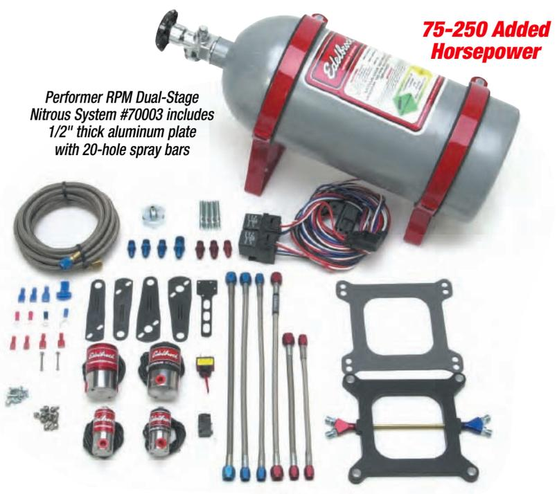
Performer RPM Dual-Stage Nitrous System #70003 includes 1/2" thick aluminum plate with 20-hole spray bars
