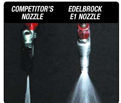
Patented E1 Nozzles deliver superior atomization using multiple radiuses to give the least amount of turbulence and a more precise spray pattern
