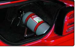
Edelbrock Nitrous Bottle installed in a 1994 Ford Mustang 5.0L
