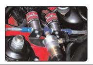
EFI Dry Nitrous Kit #70400 installed on a 1994 Ford Mustang 5.0L
