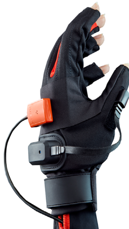
Figure 13: The Manus Xsens Glove combines IMU sensors from an Xsens suit with specialized finger sensors to provide accurate hand tracking data that correctly integrates with body data. [Image courtesy of Manus VR]
