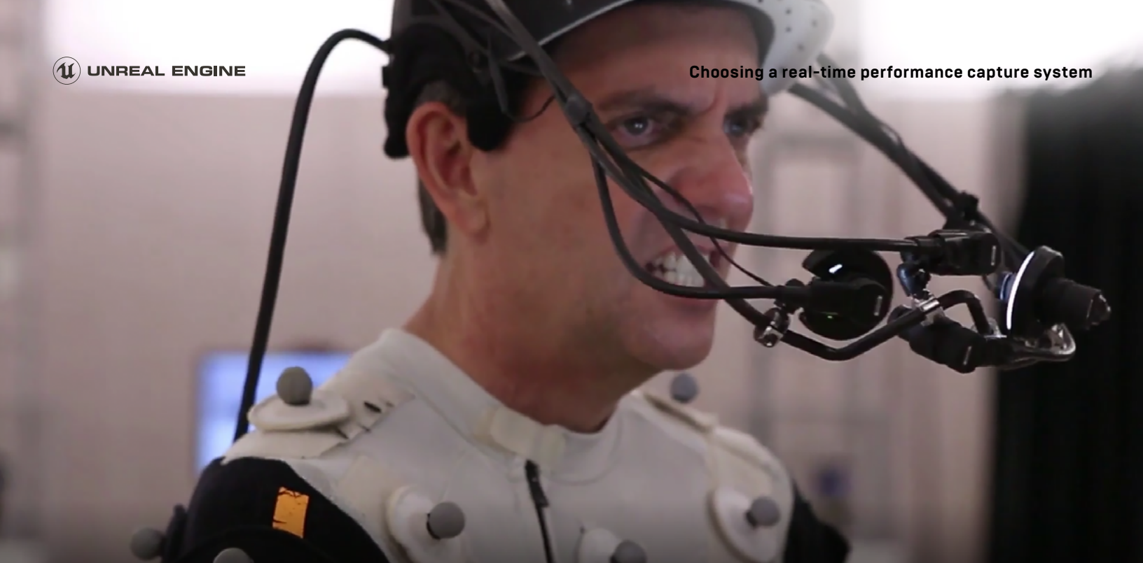
Figure 12: Doug Roble of Digital Domain using head-mounted camera for facial capture [Image courtesy of Digital Domain]
