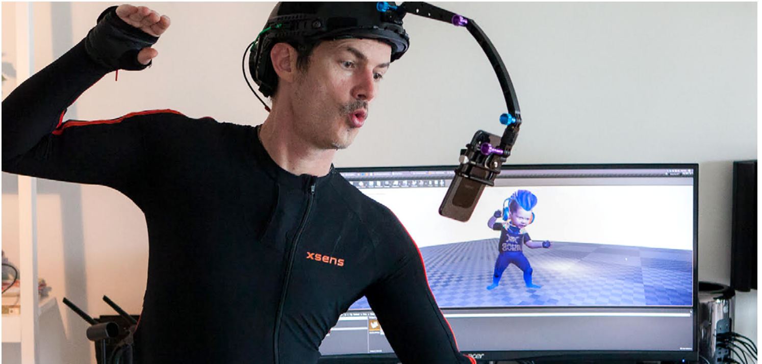
Figure 15: An iPhone X acts as a depth sensor/camera for facial capture. [Image courtesy of Kite & Lightning]
