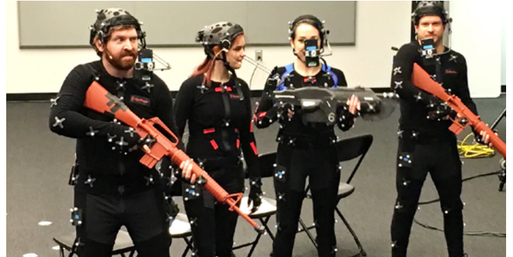
Figure 2: Mocap suits with optical passive markers used in Epic’s demonstration of virtual production techniques
