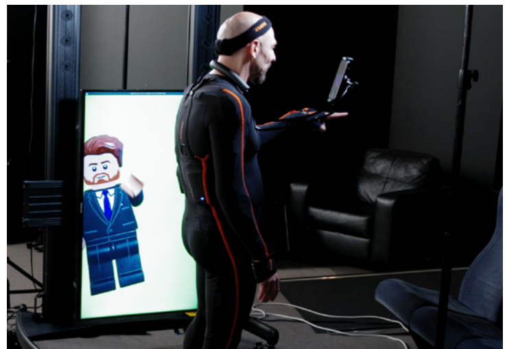
Figure 3: Inertial suit used for LEGO/HQ Trivia broadcast on mobile [Image courtesy of Animal Logic]
