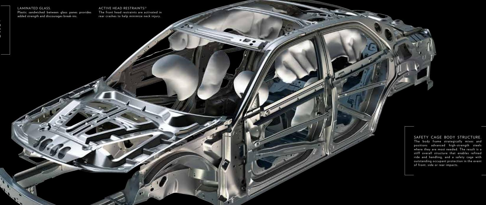
FRONT AND REAR CRUMPLE ZONES. Specially formed structural members crumple and absorb energy in a collision, helping to protect the occupant cabin. SEAT BELTS. Three-point seat belts in all five
