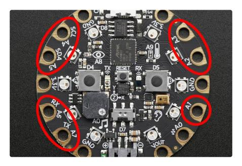
Since the pads are capacitive, you can also attach alligator clips to them and any number of capacitive items and touch those to activate them as well! For example, you could attach one end of an alligator clip to one of the pads and the other end to an apple or a lime. Or place the other end in a glass of water. Then touch the fruit or the glass of water. You'll activate the pad!
