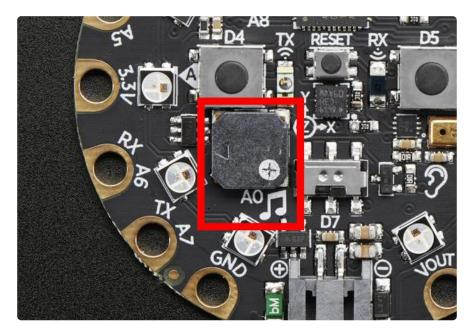
Sound files for the Circuit Playground library should be 22,050 kHz, 16-bit, mono (or less) WAV files to play on these boards. If you have an MP3 or a file you downloaded and are unsure of the encoding, you can follow this audio conversion guide () to get your files into the proper format.
