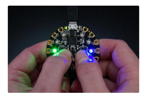
Our code is checking to see if each button is pressed. If it is, it turns on the LED next to the button to the specified color. Button A turns the LED next to it green. Button B turns the LED next to it blue. And, if the buttons are not being pressed, the LEDs are otherwise turned off by cp.pixels.fill((0, 0, 0)).
