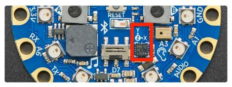
An accelerometer measures acceleration. You can read more about acceleration <a href="here">here</a>
