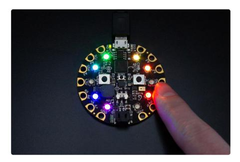
Now let's look at the code. We import time and cp. We set the LED brightness to 30%. We check to see if each pad is touched, and if it is, we print to the serial console. This time, though, we also light up a specific LED with each pad using cp.pi xels[#] = (r, g, b) where # is the pixel number and r, g, b are the color values. We didn't include any code to tell the LEDs to turn off, so they will stay on once you turn them on.
