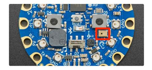
While the Circuit Playground Express also has a sound sensor, this feature of the Circuit Playground library is not available for the Express. The Express and Bluefruit have different microcontroller chips. The SAMD21 on the Express is not capable of handling the sound sensor features of the Circuit Playground Library.
