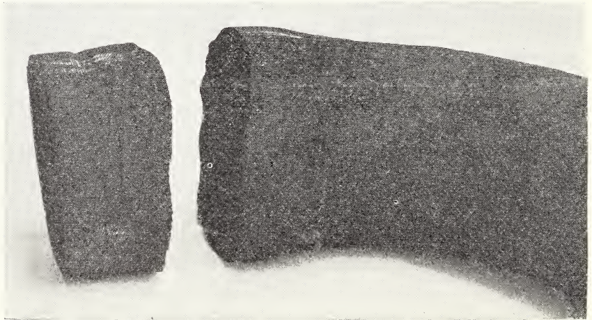
FIGURE 5. Automotive radiator hose after 7 days' use with petroleum antifreeze. Car was operated 230 miles at speeds not over 30 mph in city, in normal service, during the life of this hose.
