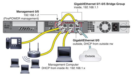
**a.** Cable Management 0/0 (for the ASA FirePOWER module) directly to one of: GigabitEthernet 0/1 through GigabitEthernet 0/5 (through 0/7 for the ASA 5525-X, 5545-X, and 5555-X).
