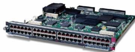
Figure 3. Cisco Express Forwarding 256 Copper 10/100 Interface Module (part number WS-X6548-RJ-45)
