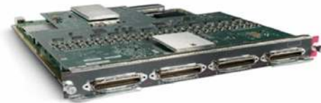
Figure 9. Cisco Classic 96-Port 10/100 (with field upgrade option to 802.3af PoE module) (part number WS-X6196-RJ-21)
