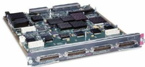
Figure 4. Cisco Express Forwarding 256 Copper 10/100 Interface Module (part number WS-X6548-RJ-21)
