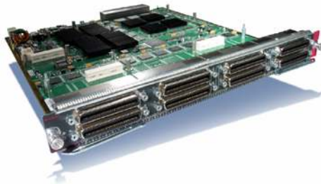
Figure 9. Cisco Classic 96-Port 10/100 (with field upgrade option to 802.3af PoE module) (part number WS-X6196-RJ-21)
