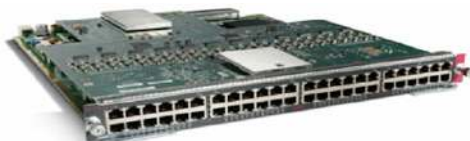
Figure 7. Cisco Classic 48-Port 10/100 802.3af PoE Module (part number WS-X6148A-RJ-45)
