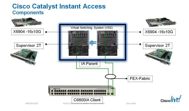
The Cisco Cat 3560CX-12PD-S or Cisco Cat 3560CX-8XPD-S can replace the C6800IA client in the configuration depicted in the figure above. The list of line cards that are supported on the IA Parent switch in the IA Parent-Child connection is restricted to – WS-X6904-40G, C6800-32P10G-XL, C6800-16P10G-XL and C6800-8P10G-XL.
