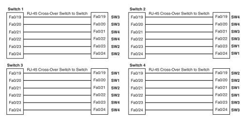
Figure 1-2 Switch Cabling
