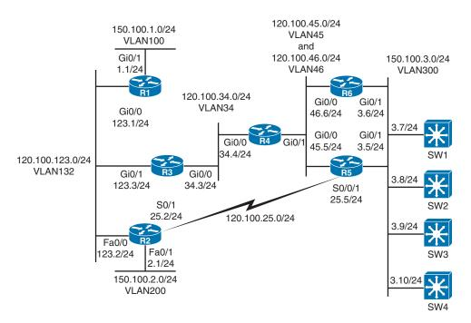
Figure 1-3 IP Addressing Diagram
