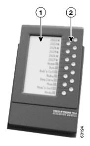
1 Phone screen—Displays the phone number, speed dial number (or name or other text label), phone service, or Privacy assigned to each button. Icons indicating line status appear and function the same as those on the Cisco IP Phone 7960G to which it is attached.
