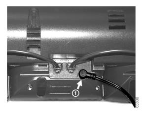
Power supply connector on the back of the Expansion Module
