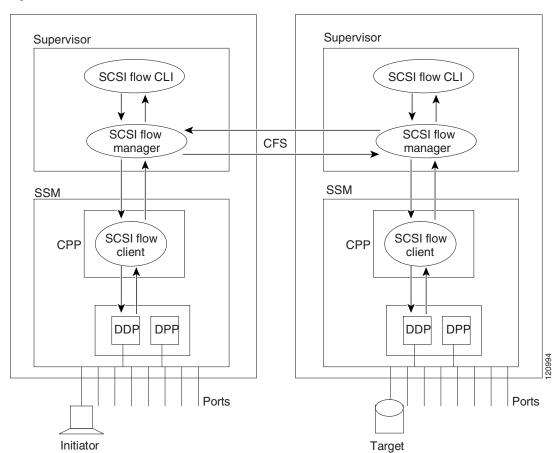
Figure 2-1 SCSI Flow Services Functional Architecture
