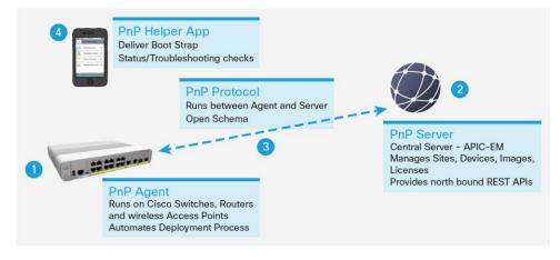
Figure 1. Cisco Plug and Play Solution Components
