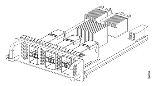
Figure 1-36 Front View of the N5K-M1060 GEM
