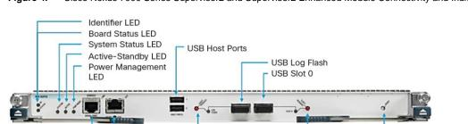
Figure 4. Cisco Nexus 7000 Series Supervisor2 and Supervisor2 Enhanced Module Connectivity and Indicators
