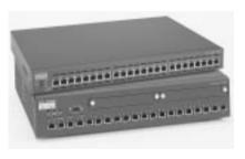
The Catalyst 3900 is a stackable switch that offers 20 fixed ports, a stack port, and a unique FlexSlot that supports one double-wide card or up to two feature cards that can provide additional Token Ring ports or high-speed uplinks. The Catalyst 3920 offers 24 fixed Token Ring ports and can be stacked with other Catalyst 3920 units or with the Catalyst 3900.
