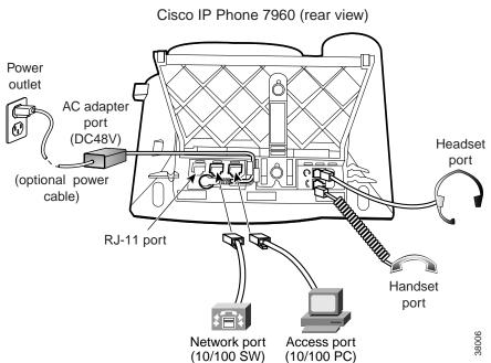
Figure 1-3 Cisco SIP IP Phone Cable Connections
