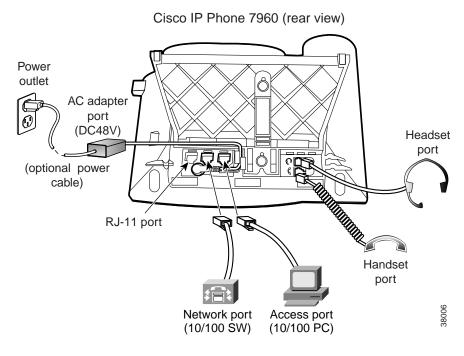
Figure 2-1 Cisco SIP IP Phone Cable Connections
