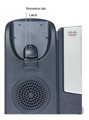
**STEP 3** Rotate the tab 180° and re-insert into the phone base. The tab now catches the slot in the handset when the handset is placed onto the cradle.
