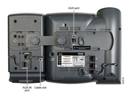
**STEP 10** Route the auxiliary cable inside the cable slot of the Cisco SPA 500S.
