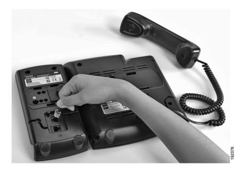
STEP 7 Locate the AUX port on the back of the SPA525G. Connect the other end of the auxiliary cable to this port.
