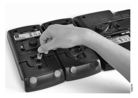
**STEP 7** Route the auxiliary cable inside the cable relief channel.
