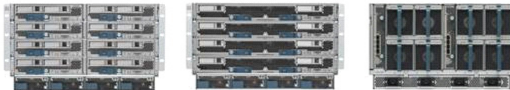
Figure 4 Cisco UCS 5108 Blade Server Chassis with Blade Servers Front and Back
