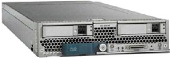
Figure 3 Cisco UCS B200 M3 Blade Server
