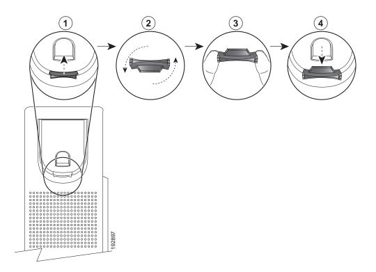
1 Remove the handset from the cradle and pull the plastic tab from the handset rest.
