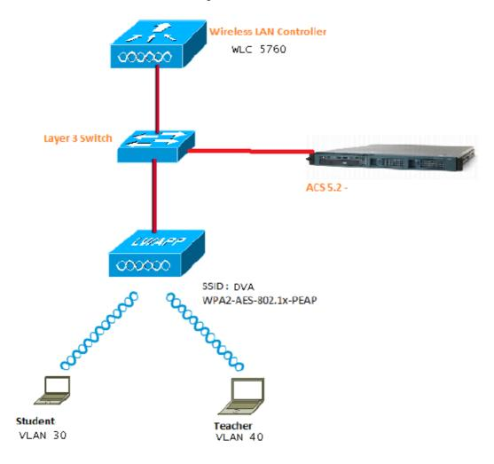
This document uses 802.1X with Protected Extensible Authentication Protocol (PEAP) as the security mechanism.
