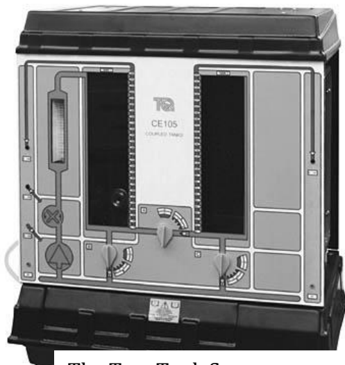
The Two Tank System
