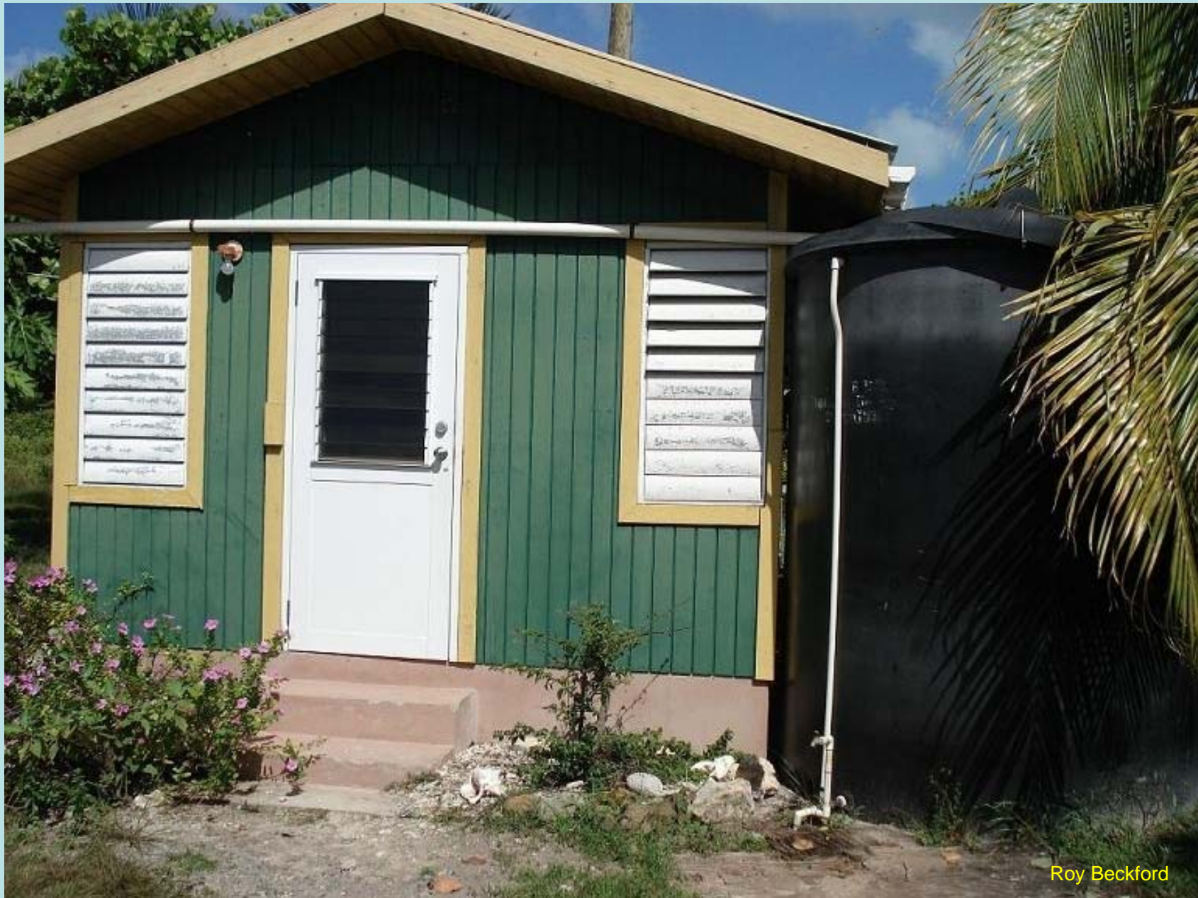
A rain barrel used to collect rain water from the roof. It supplies irrigation water to a 1.0 acre small farm.
