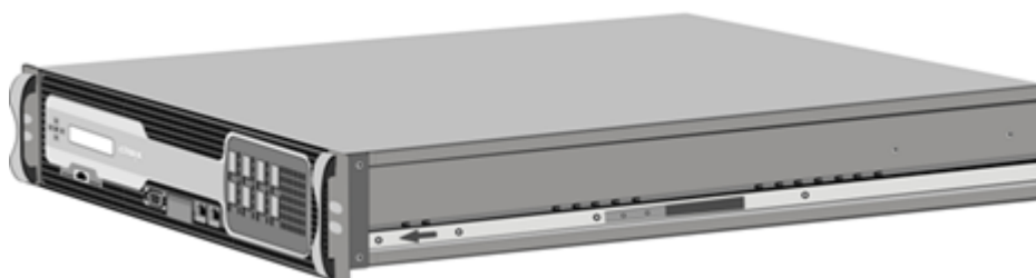
Figure 1. Attach inner rails
