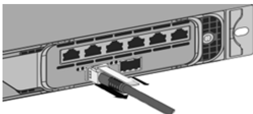
Figure 9. Remove a DAC from the 10G port
