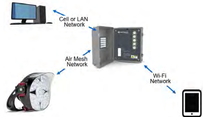
Example LED Field Lighting System
