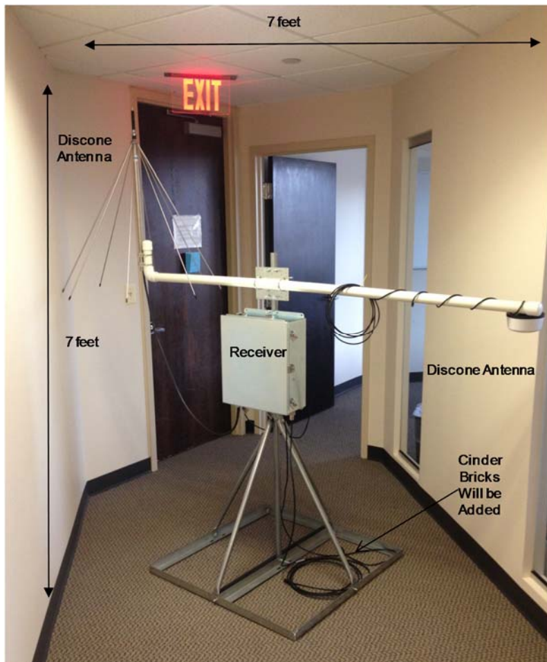
Figure 1: Typical configuration of CityScope station sensor.
